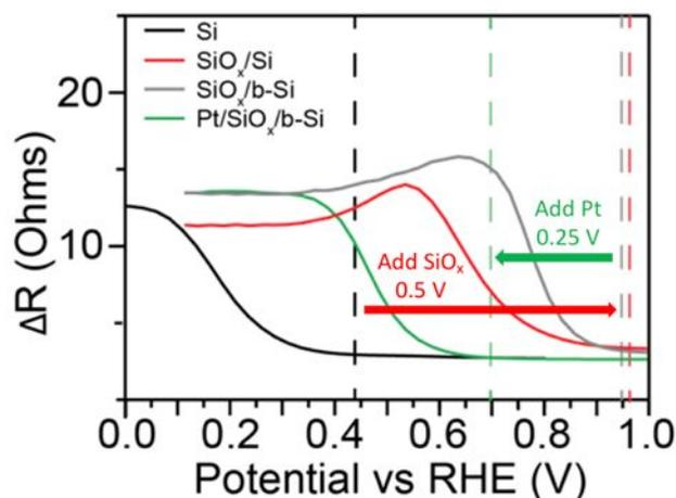
Fig. 5 The thermodynamic flatband potential  $U_{fb}$  measured by intensity-modulated high frequency resistivity (IMHFR) spectroscopy at p-type Si electrodes shifts from the bare, hydrogen-terminated Si surface to more positive potentials as an oxide layer is formed
