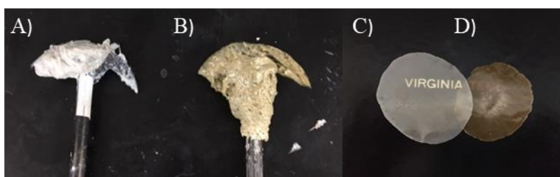
Figure 1. Poly(hydroquinone-3,4'-bibenzoate) before (A/B) and after (C/D) compression molding utilizing hydroquinone dipivilate (A/C) or hydroquinone diacetate (B/D).
