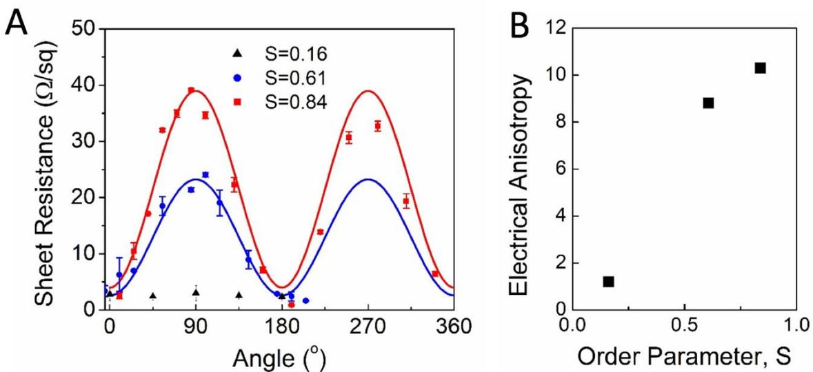
Fig. 3: Angle-dependent sheet resistance of the AgNW coatings. (A) Sheet resistance as a function of measurement angle relative to the alignment of the AgNW coatings (*i.e.*, with order parameters of 0.84, 0.61, 0.16). Solid lines are fits to a sinusoidal function; (B) Electrical anisotropy as a function of order parameter.
