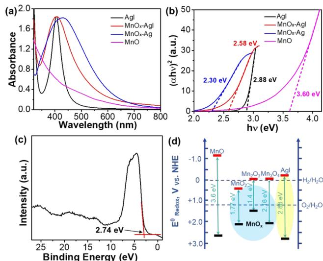
**Figure 4.** The band gap and electronic analysis of Janus-type MnO<sub>x</sub>-AgI NPs. (a) The UV-Vis spectra and (b) Tauc plots of AgI (black), MnO octahedra (pink), MnO<sub>x</sub>-Ag (blue) and MnO<sub>x</sub>-AgI NPs (red). (c) Valence-band XPS spectrum of AgI NPs. (d) The scheme to show the proposed realignment of the conduction band and valence band of Janus-type MnO<sub>x</sub>-AgI NPs.
