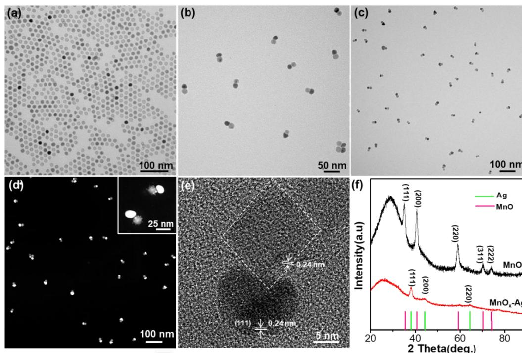
**Figure 1.** The growth and characterizations of Ag domains on MnO octahedra. (a) Low-magnification TEM image of MnO octahedra. (b-c) TEM (d) HAADF-STEM and (e) HR-TEM images of Janus-type  $\text{MnO}_x$ -Ag NPs. (f) Powder XRD patterns of MnO octahedra (black, top) and  $\text{MnO}_x$ -Ag (red, bottom). The diffraction peaks for pure Ag and MnO are indicated by vertical lines at the bottom using JCPDF#4-783 and JCPDF#72-783, respectively.
