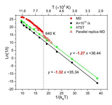
Figure 8. Arrhenius plots for the  $n=0\rightarrow 1$  transition obtained from MD and AKMC simulations. The black and the green dots represent data from AKMC simulations with  $A=10^{13}/s$  and explicitly calculated from hTST ( $A = \frac{\prod_{i}^{3N} v_i^{init}}{\prod_{i}^{3N-1} v_i^{\frac{1}{2}}}$ ), respectively. The red circles and triangles are computed with conventional MD and parallel replica MD simulation, respectively.
