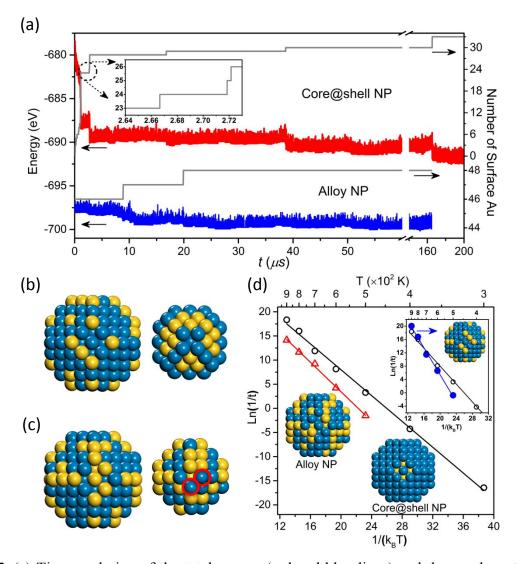
**Figure 5.** (a) Time evolution of the total energy (red and blue lines) and the number of surface Au atoms (grey lines) for AKMC simulations of the  $Au_{79}@Pd_{122}$  core@shell (upper panel) and random alloy (lower panel) NP at 800 K. To show the escape process from the n=24 state, the
