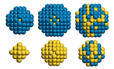
**Figure 1.** Geometric structures of PdAu NP models used in this study,  $Au_{19}@Pd_{60}$  and  $Au_{79}@Pd_{122}$  core-shell and  $Au_{79}Pd_{122}$  random alloy. The lower panel shows the corresponding core structure of each model, with the surface atoms removed. The blue and the gold spheres represent the Pd and the Au atoms, respectively. The same color code is used for all subsequent figures.
