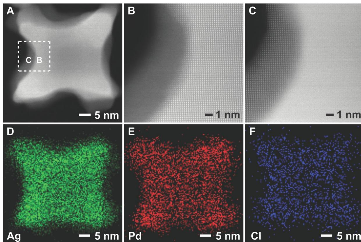
**Figure 2.** (A-C) HAADF-STEM images of a sample prepared with the addition of 0.4 mL of the Pd(II) precursor solution (see Figure 2E). (D-F) EDX elemental mapping of the same sample (green: Ag; red: Pd; blue: Cl).
