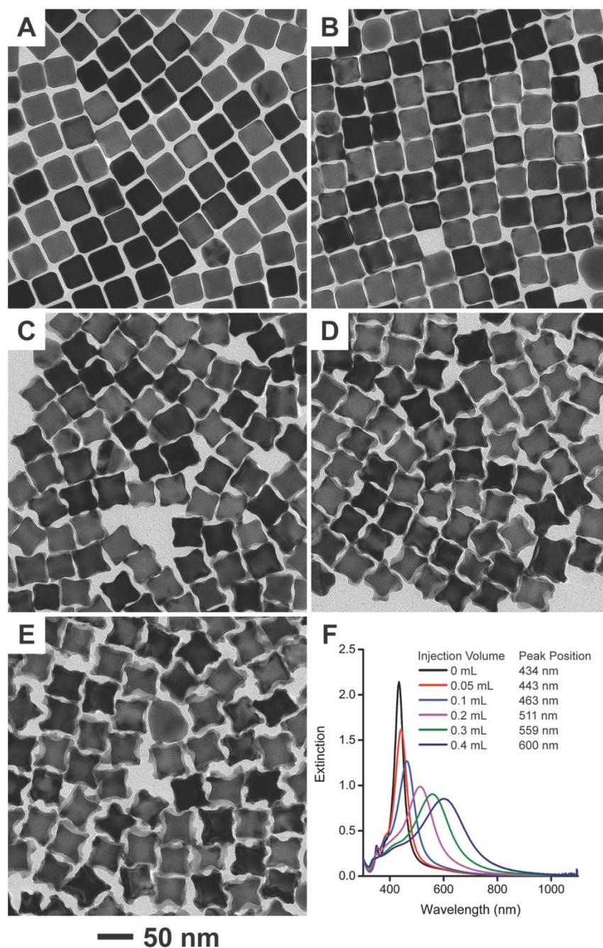
**Figure 1.** TEM images of concave nanocrystals prepared by reacting Ag nanocubes with different volumes of the Pd(II) precursor solution: (A) 0.05 mL, (B) 0.1 mL, (C) 0.2 mL, (D) 0.3 mL, and (E) 0.4 mL, respectively, in the presence of CTAC. (F) UV-vis spectra of Ag nanocubes before and after reacting with different volumes of the Pd(II) precursor solution.
