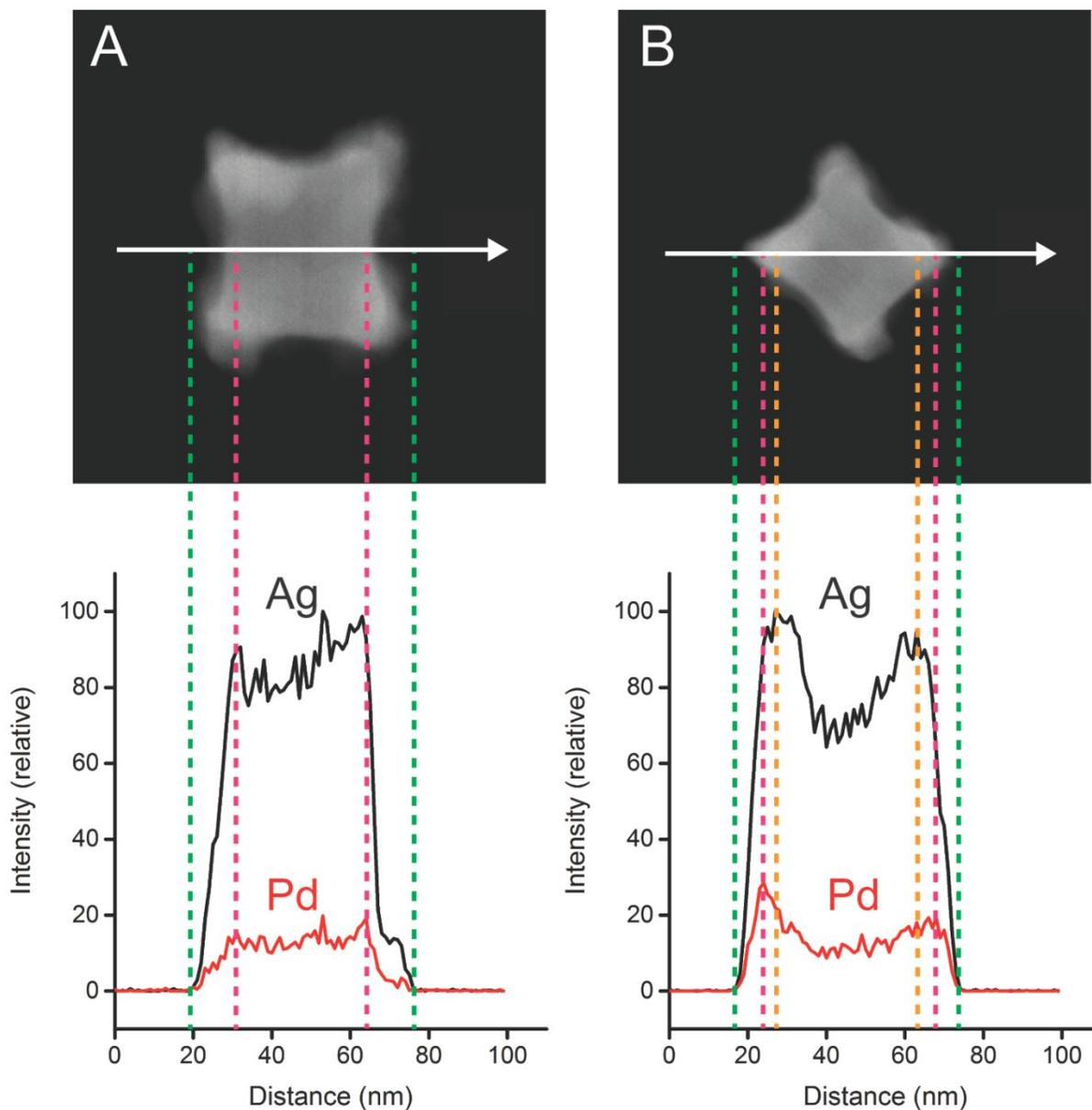
**Figure 3.** (A) A HAADF-STEM image taken from an individual concave nanocrystal prepared with 0.4 mL of the Pd(II) precursor solution and the corresponding EDS line-scan results. (B) A HAADF-STEM image taken from the same particle in (A) but with the raster angle rotated by 45 degrees and the corresponding EDS line-scan data. The particle was oriented along the  $\langle 001 \rangle$  zone axis.
