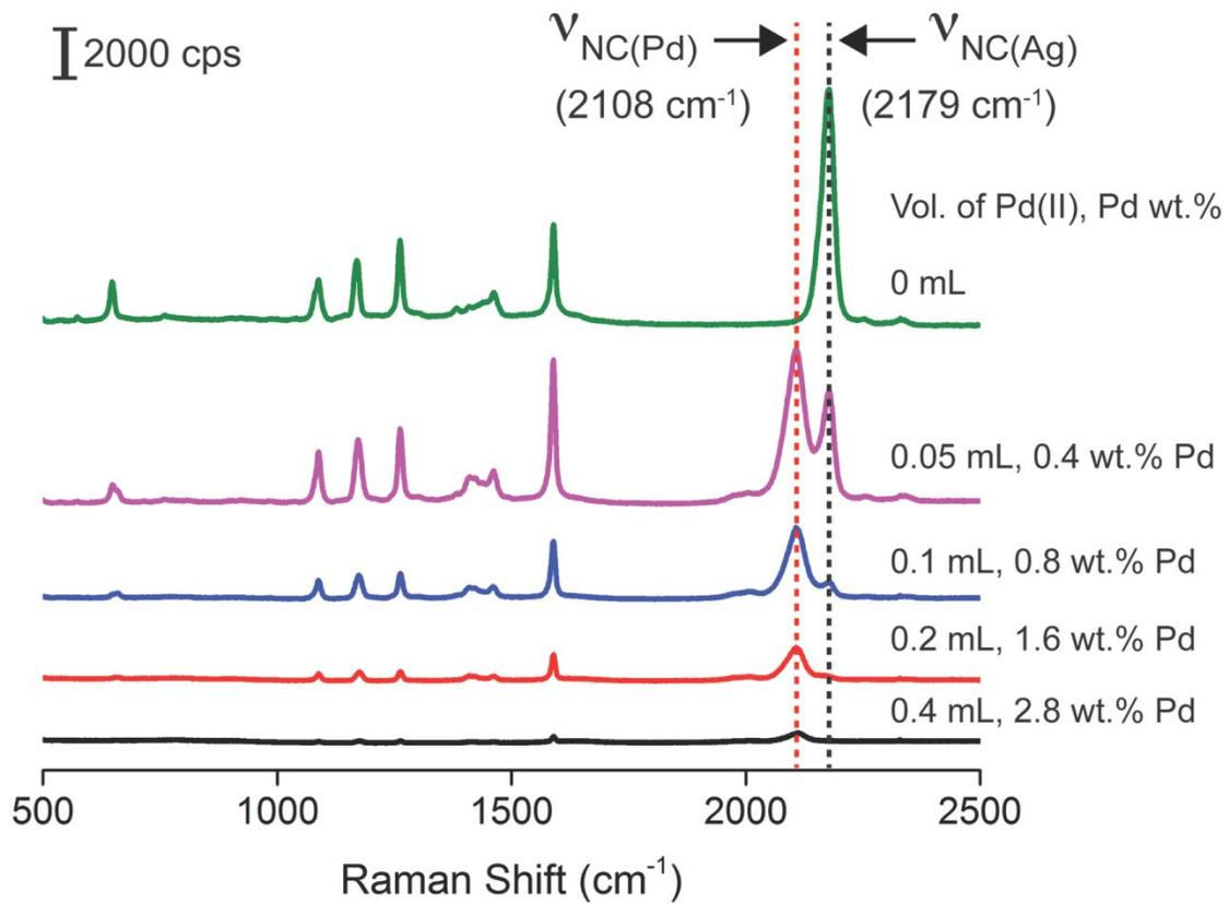
**Figure 6.** SERS spectra recorded from the CTAC-treated, 2,6-DMPI-functionalized Ag nanocubes and the Ag-Pd nanocrystals prepared with different volumes of the Pd(II) precursor solution.
