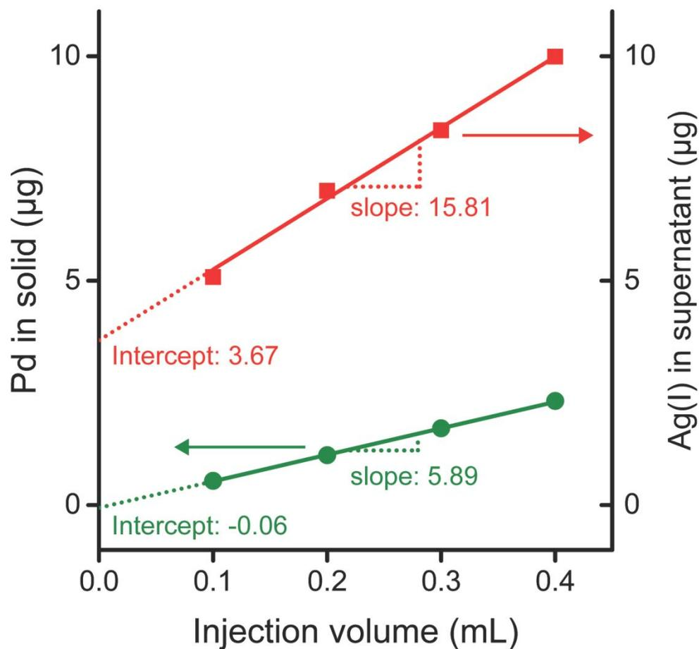
**Figure 5.** ICP-MS data of Pd in solids and Ag(I) in supernatant for the corresponding products prepared by introducing different volumes of the Pd (II) precursor solution into an aqueous suspension of Ag nanocubes in the presence of CTAC.
