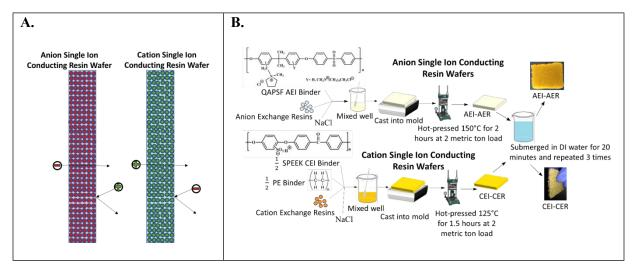
Figure 2. (a) Illustration of single ion-conducting RWs. (b) Manufacturing scheme for single anion- and single cation-conducting RWs.
