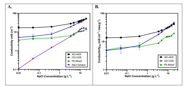
**Figure 3. (a)** Ionic conductivity of single ion-conducting RWs at various NaCl concentrations. **(b)** Ionic conductivity normalized to ion-exchange capacity at various NaCl concentrations. Error bars in these plots represent the absolute difference (n=2) from the average for the ionomer RWs.
