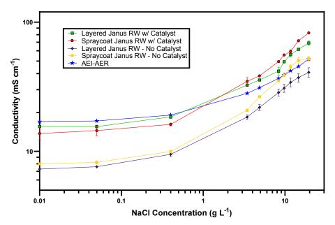
**Figure 7.** Ionic conductivity of symmetric and asymmetric Janus bipolar RWs with and without water dissociation catalyst. Error bars represent absolute difference (n=2) from the average of measurements.
