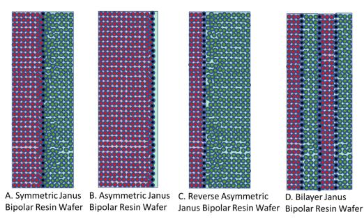
**Figure 4**. Cross-sectional views of (a) symmetric and (b) asymmetric Janus bipolar resin wafers used in this report and concepts of a (c) reversed asymmetric and (d) bilayer Janus bipolar resin wafer.
