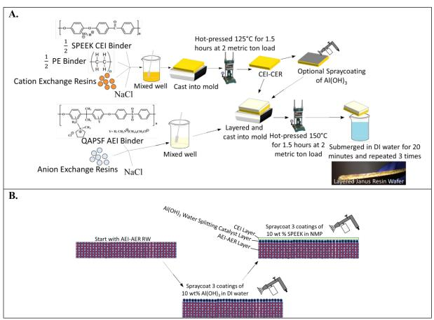
**Figure 5. (a)** Manufacturing scheme for symmetric Janus bipolar RW with optional inclusion of a water dissociation catalyst (Al(OH)<sub>3</sub> nanoparticles). **(b)** Manufacturing scheme for an asymmetric Janus bipolar RW with optional inclusion of a water dissociation catalyst.
