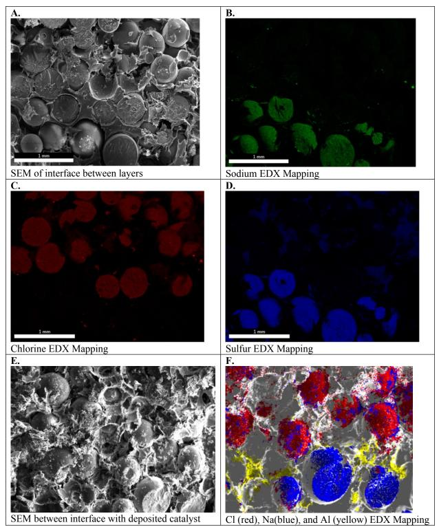
**Figure 6.** Electron micrographs of symmetric Janus bipolar RW interface without a catalyst (a) Image with no EDX mapping. (b) Chlorine (Cl) EDX map (anion exchange layer). (c) Sodium (Na) EDX map (cation exchange layer). (d) Sulfur EDX map. Electron micrographs of symmetric Janus bipolar RW interface (e) image without EDX mapping and (f) EDX mapping of Cl, Na, and aluminum (Al).
