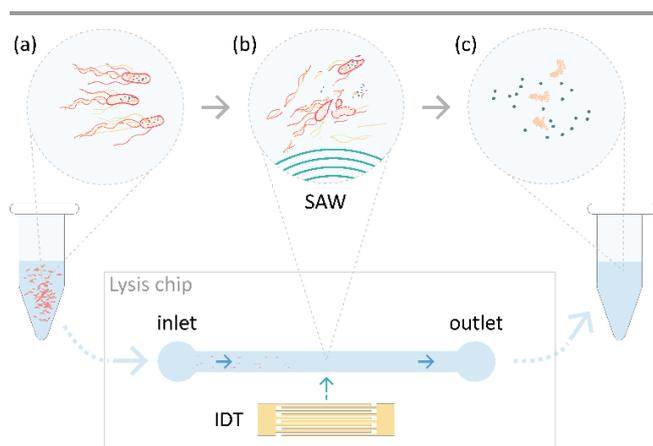
**Fig. 1** Overview of the TSAW lysis device (top view). The lysis chip consists of a PDMS microchannel plasma-bonded to a lithium niobate ( $\text{LiNbO}_3$ ) substrate with an interdigitated transducer (IDT) adjacent to the microchannel to generate traveling surface acoustic waves. We flow the bacteria suspension through the microchannel (a) at a constant flow rate, expose the bacteria suspension to a TSAW field at 33.3% duty cycle (b) and collect the lysate for further analysis (c).
