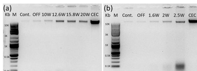
**Fig. 5** Agarose gel electrophoresis analysis of nucleic acids extracted at indicated TSAW power level. (a) Traveling surface acoustic waves at frequency of 13 MHz. (b) Traveling surface acoustic waves at frequency of 160 MHz. The no-lysis control ("Cont.") is generated from bacteria kept on ice. The Complete Extraction Control ("CEC") is prepared using the Bacterial Genomic DNA Kit. "M" is 100 bp DNA ladder; "Kb" is Kilobases.
