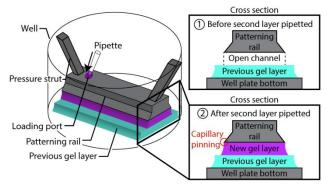
**Figure 1.** Schematic showing the mechanism of layer-by-layer gel patterning using open microfluidics. An open channel is created above an existing gel layer using a rail-based patterning device.
