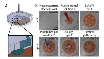
**Figure 5.** Integrated fluidic channels in patterning device for depositing second material in a layer. (A) Cross-sectional schematic representation of 'void-filling' patterning device with underlying layer. (B) Video stills of patterning red colored agarose (250  $\mu$ m thick) and filling voids with blue colored agarose (750  $\mu$ m thick). Full video available in the SI.
