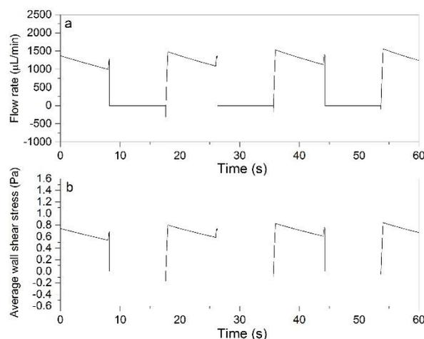
**Figure 4:** Calculated flow rates and shear inside the microfluidic channels during device operation.
