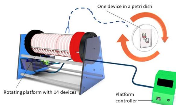
**Figure 3:** Rotating platform. Microfluidic devices are placed in petri dishes and placed vertically into the platform. The platform holds up to 14 petri dishes. For this study we rotated the petri dishes by 180° every eight-seconds. Details of the fluidic device are shown in Fig. 1.
