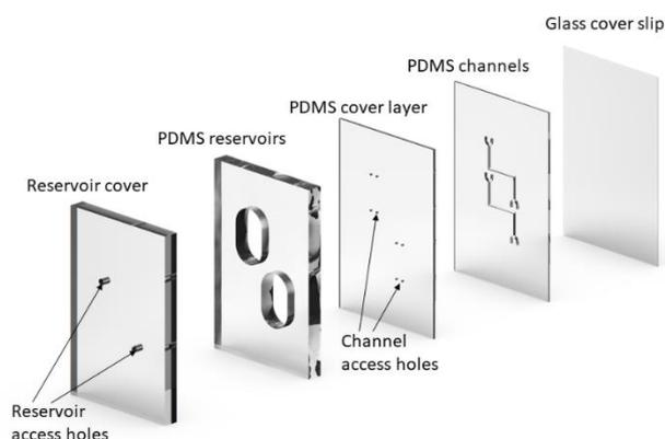
**Figure 1:** Layers of the microfluidic device. The device consists of a thin glass layer and several PDMS layers. A key feature of the design are the channel access holes through which cell culture medium can leave the upper reservoirs to flow into the lower reservoir. To create unidirectional flow it is important that the channel access holes are placed at the top and bottom region of the reservoir, and at least 1 mm away from the reservoir walls.
