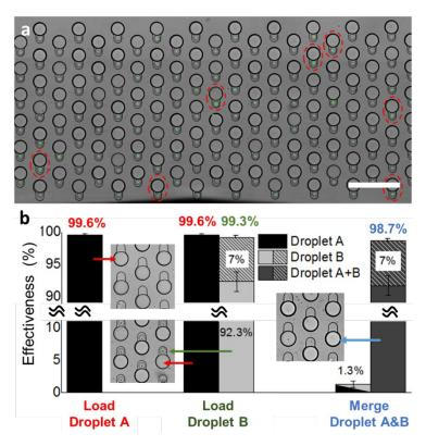
**Figure 6. Quantification of the merging device effectiveness.** (a) Image of paired droplets in a droplet storage array. The dashed circles indicate there are multiple cells in single droplet Bs. (b) Effectiveness for droplet trapping, pairing, and merging steps. The slash bars indicate the percentage of droplets containing more than one cell.
