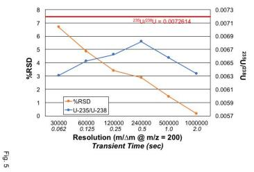
Figure 5. Effect of increasing mass resolution setting (specified at m/z = 200 Da) on the accuracy and precision of the  $^{235}$ U/ $^{238}$ U isotope ratio measurement. Each data point represents 3 acquisitions, each of which consisted of 10 scans of 10 microscans. CRM 129a test solution = 100 ng mL<sup>-1</sup>. Conditions: discharge current = 30 mA, solution flow rate = 30  $\mu$ L min<sup>-1</sup>, and sheath gas flow rate = 0.5 L min<sup>-1</sup>.
