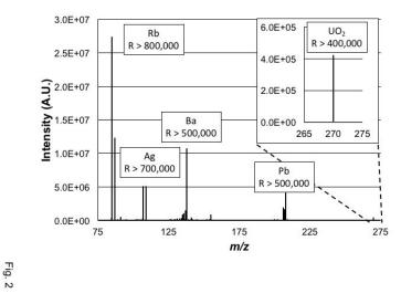
Figure 2. Representative mass spectrum of a multi-element solution containing 500 ng mL<sup>-1</sup> each of Rb, Ag, Ba, Pb and U. The spectrum was taken in 'full scan' mode using a resolution setting of 500,000, specified for m/z = 200 Da. Conditions: discharge current = 30 mA, solution flow rate = 30  $\mu$ L min<sup>-1</sup>, and sheath gas flow rate = 0.5 L min<sup>-1</sup>.
