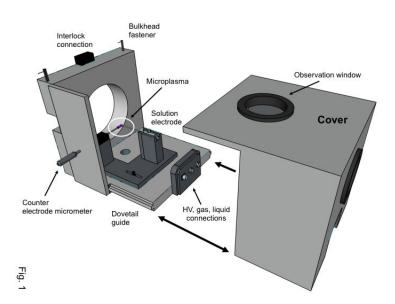
Figure 1. Expanded view of the new LS-APGD ion source housing and components.
