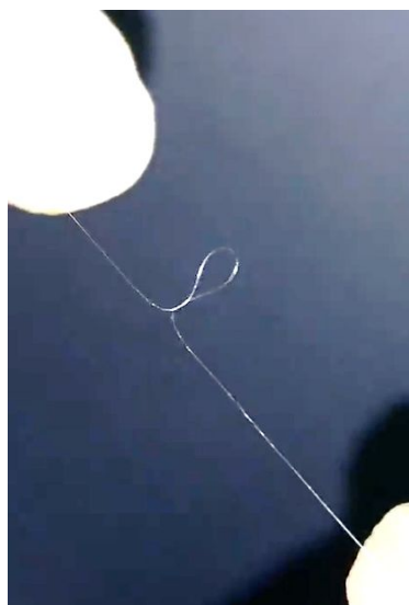
Figure 5 Keratin filament endured a high degree of twisting.
