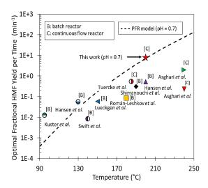
Microreactors enable the highest yields of HMF at ultrashort reaction times to increase HMF productivity by 10- to 1000-fold.
