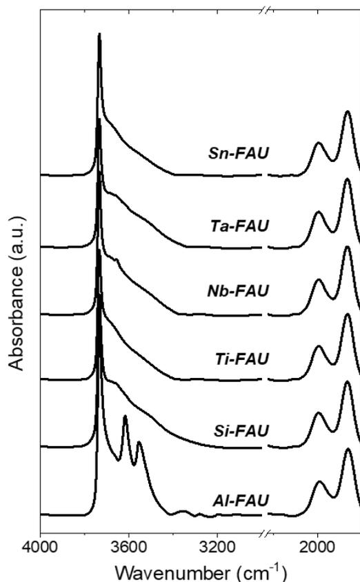
**Figure 5.** Infrared spectra of dehydrated Al-, Si-, Ti-, Nb-, Ta-, and Sn-FAU in flowing He (50 cm<sup>3</sup> min<sup>-1</sup>, 573 K). Spectra have been normalized to  $\nu(\text{Si-O-Si})$  at 1865 cm<sup>-1</sup> and are vertically offset for clarity.
