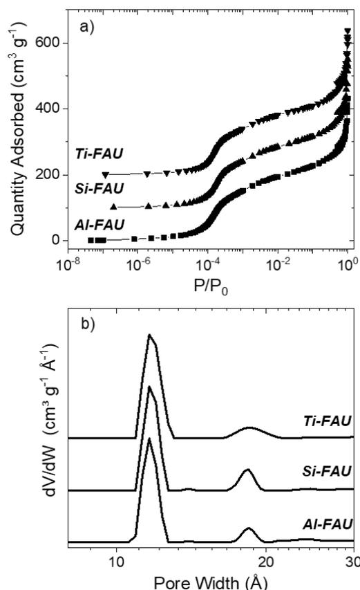
**Figure 2.** (a) Nitrogen adsorption isotherms (77 K; offset by  $100 \text{ cm}^3 \text{ g}^{-1}$  for clarity) and (b) pore-size distributions for Al-FAU, Si-FAU, and Ti-FAU. The pore-size distributions were calculated using a cylindrical pore model with NLDFT. Pore-size distributions are normalized to the 1.15 nm feature and offset for clarity.
