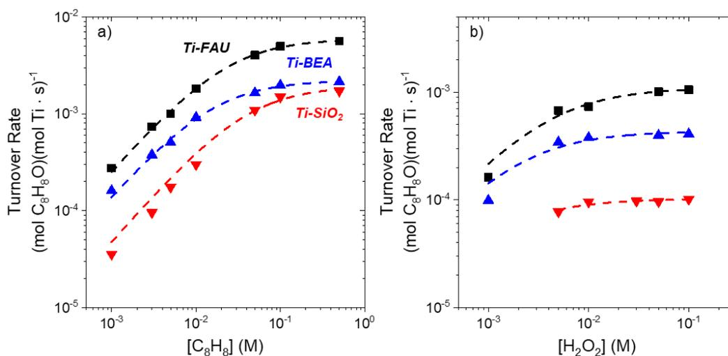
**Figure 8.** Turnover rates for  $C_8H_8$  epoxidation as a function of (a)  $[C_8H_8]$  ( $0.01\text{ M } H_2O_2$ ) and (b)  $[H_2O_2]$  ( $3 \cdot 10^{-3}\text{ M } C_8H_8$ ) on Ti-FAU (black ■), Ti-BEA (blue ▲), and Ti-SiO<sub>2</sub> (red ▼) in  $CH_3CN$  at 313 K. Dashed lines represent fits to equation 4. Data for Ti-BEA and Ti-SiO<sub>2</sub> are adapted from ref 23. Errors in  $C_8H_8O$  formation rates are <10% and error bars are omitted for clarity.
