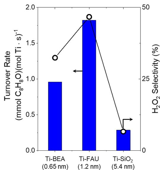
**Figure 7.** Turnover rates for  $\text{C}_8\text{H}_8$  epoxidation (blue bars) and  $\text{H}_2\text{O}_2$  selectivities towards epoxidation products (black o) over Ti-BEA, Ti-FAU, and Ti-SiO<sub>2</sub> with the characteristic pore dimension indicated. All reactions were run at standard conditions that lead to rates that are proportional to  $\text{C}_8\text{H}_8$  concentrations (0.01 M  $\text{C}_8\text{H}_8$ , 0.01 M  $\text{H}_2\text{O}_2$  in  $\text{CH}_3\text{CN}$ , 313 K).
