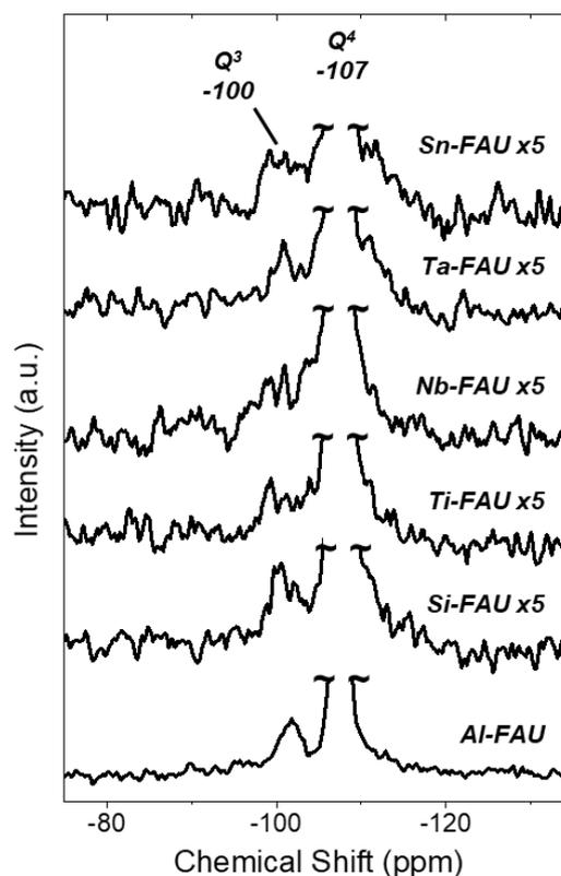
**Figure 4.**  $^{29}Si$  direct polarization MAS-NMR spectra of Al-, Si-, Ti-, Nb-, Ta-, and Sn-FAU. Spectra are normalized to the  $Q^4$  feature and scaled to the indicated value (e.g., x5 magnification for Si-FAU). The intense  $Q^4$  feature has been truncated and spectra are vertically offset for clarity. Figure S5 shows  $^{29}Si$  MAS-NMR spectra that includes the  $Q^4$  feature.
