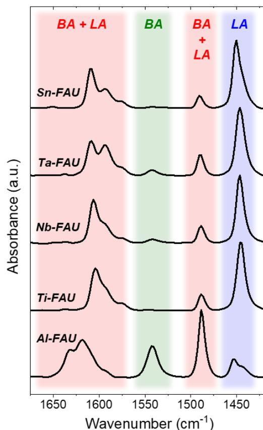
**Figure 6.** Infrared spectra of Al-FAU, Ti-FAU, Nb-FAU, Ta-FAU, and Sn-FAU in contact with gaseous pyridine (0.25 kPa, 101 kPa He, 473 K). All spectra were normalized to the most-intense feature between 1700 – 1400  $\text{cm}^{-1}$  and are offset for clarity. Colored regions correspond to expected regions for vibrational modes of pyridine coordinated to Lewis acid sites (LA; blue), Brønsted acid sites (BA; green), and both Brønsted and Lewis acid sites (BA + LA; red).
