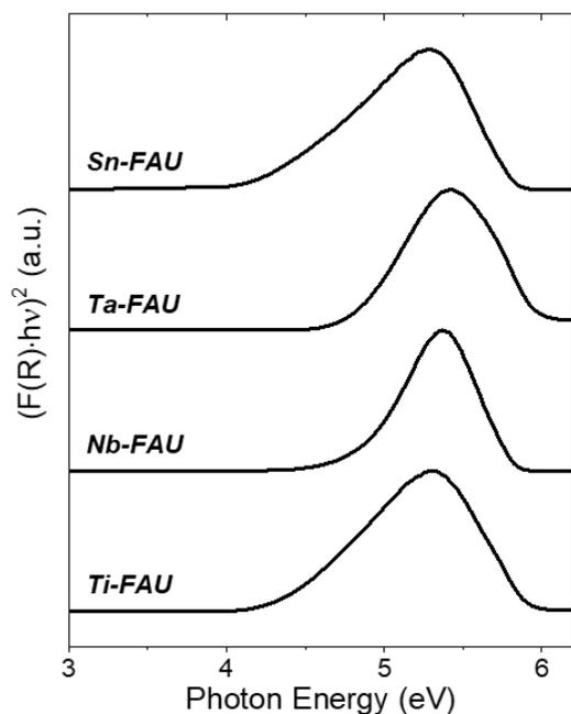
**Figure 3.** Tauc plots for Ti-, Nb-, Ta-, and Sn-FAU. Note that  $F(R)$  corresponds to the Kubelka-Munk pseudo-absorbance. All spectra were normalized to the most-intense feature and are offset for clarity. Optical band gaps were calculated from regressing the linear portion of the leading edge to a value of zero.
