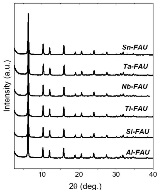
**Figure 1.** X-ray diffractograms for Al-, Si-, Ti-, Nb-, Ta-, and Sn-FAU. Diffractograms are vertically offset for clarity.
