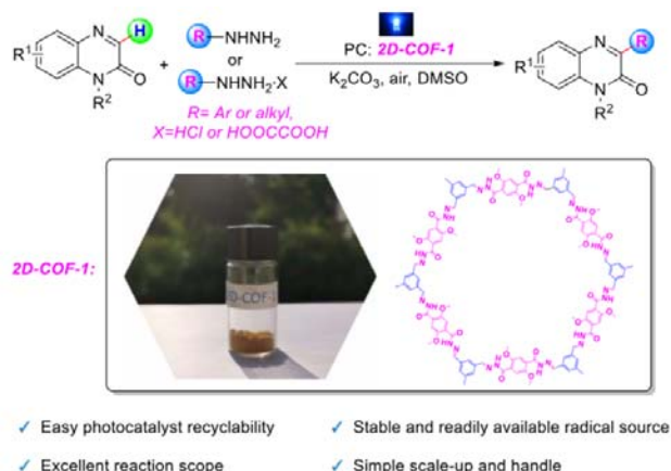
Fig. 27 The use of 2D-COF 1 as a photocatalyst for the direct C3 arylation and alkylation of quinoxalin-2(1 H )-ones. Adapted with permission from Chem. Eur. J. 10.1002/chem.201903523.
