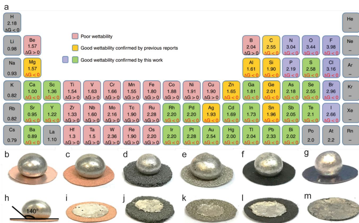
Fig. 11 a) The electronegativities, wettability and \Delta G of various elements. The wettability behaviour between molten-Li and various substrates: b) Cu, c) Cu-foam, d) Fe-foam, e) Ni-foam, f) carbon fibre and g) GO; h) The contact angle is \sim 140^\circ on the Cu surface, the interfacial wettability of i) Cu-foam, j) Fe-foam, k) Ni-foam, l) carbon fiber and m) GO are improved via abietic resin-coated substrates. 116 a-m) Reproduced with permission from ref. 116. Copyright 2019, Nature Publishing Group.
