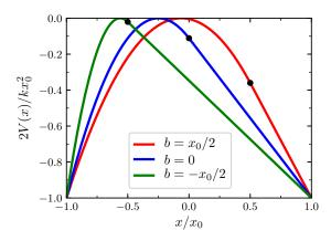
**Fig.** 1 Plot of the rescaled potential  $2V(x)/kx_0^2$  vs. rescaled distance  $x/x_0$  defined by Eq. (1) for  $b=x_0/2$ , b=0 and  $b=-x_0/2$ . The symmetric parabolic potential corresponds to  $b=x_0$  and, as the parameter b decreases, the potential becomes increasingly asymmetric. V(x) is parabolic for  $-x_0 \le x \le b$  and linear for  $b \le x \le x_0$ .
