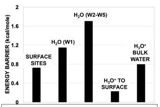
Figure 6. PMF calculations of the average energy barriers to proton transfer for transfer between silica surface sites, neutral water molecules in W1 and in W2-W5 'layers',  $H_3O^+$  ions in W1 transferring to a surface site, and  $H_3O^+$  ions transferring protons in bulk water, all at 2.4Å O-O spacing.
