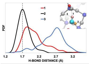
Figure 10. Labeled H-bond lengths for  $H_2O$  molecule shown in inset and figure 9 showing asymmetric H-bonds. H-bond labeled 2 shorter than normal H-bond in water (1.70Å peak max) vs.1.8 Å for water).
