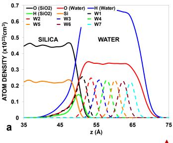
Figure 2. (a) Density profiles of atoms in the glass and water; Wi indicate location of the O atoms in water as a function of water 'layer' based on H-bonding (see text). (b) side view of system with Si atoms in blue, SiO bonds in grey, and water OH bonds in cyan; (c) SiO bonds at z>49Å and z<38 Å and water oxygen at z<49Å shown as cyan spheres. (c) shows water penetrating 11 Å below outer Si atoms at 300K.
