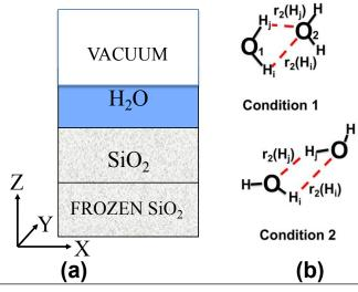
Figure 1. (a) Schematic drawing of system. (b) Conditions for describing H-bonds.
