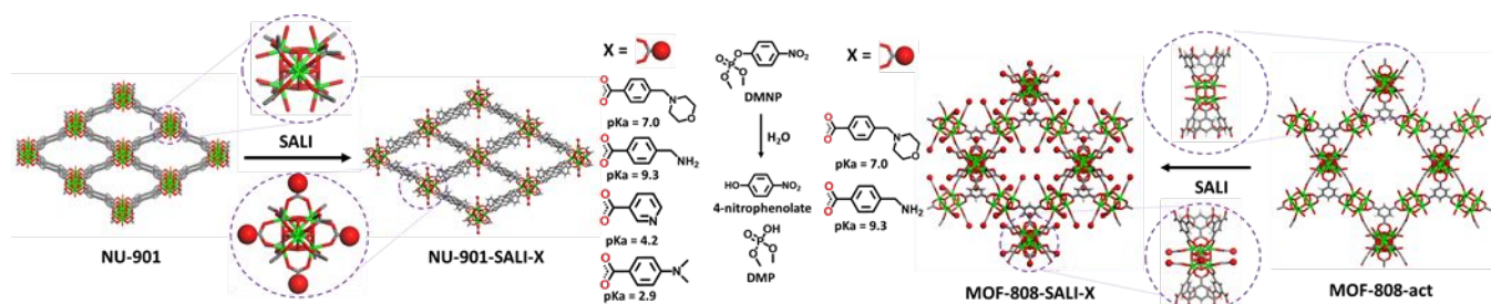
Scheme 1. Solvent-assisted linker incorporation (SALI) of amine functionalized modulators within NU-901 and MOF-808 utilized for the hydrolysis of organophosphorous compounds in pure water. pKa values were calculated through Chemicalize (ChemAxon).
