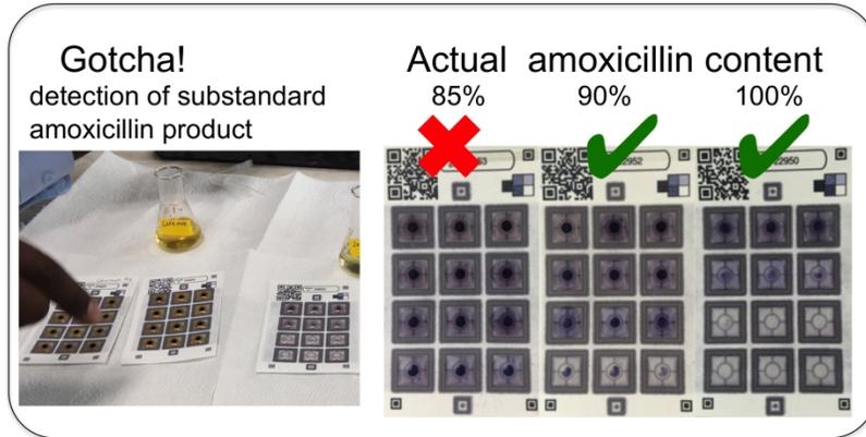
A paper analytical device can detect substandard ampicillin or amoxicillin capsules in low-resource settings.
