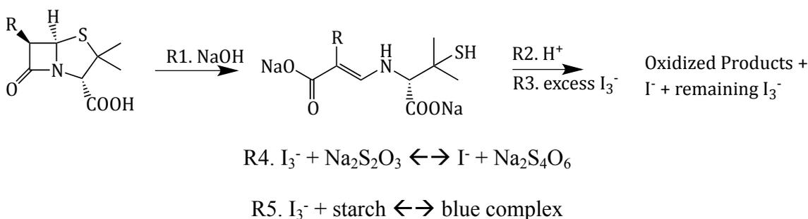
Figure 1. Back-titration of beta-lactam antibiotics. R1. The antibiotic is degraded with base to produce redox active species, reaction time = 15 min. R2. The solution is acidified. R3. A known excess of triiodide is added, reaction time = 15 min. R4. The remaining triiodide is quantified via iodometric titration. R5. The starch indicator will be colored blue if the oxidizing capacity of the triiodide exceeds the reducing capacity of the thiosulfate. If not, the indicator will be colorless.
