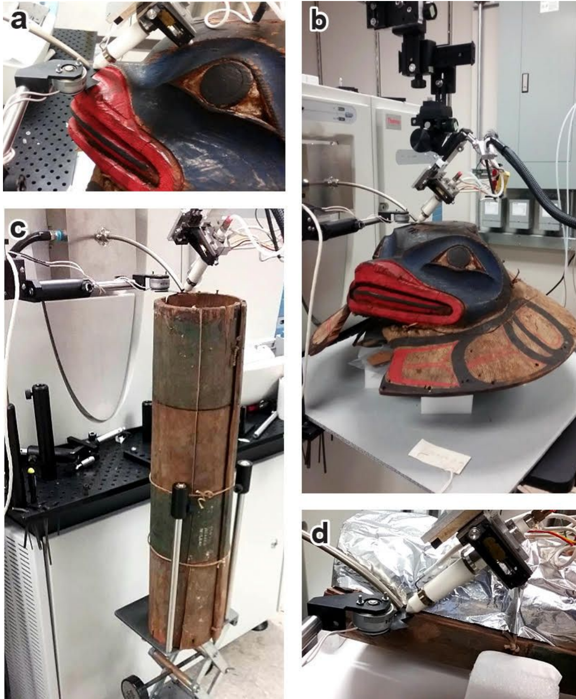
Figure 2. Reflection mode DART sampling configurations with extended transfer tube and shutter for selected surfaces on hat (a, b) and cylinder (c, d).
