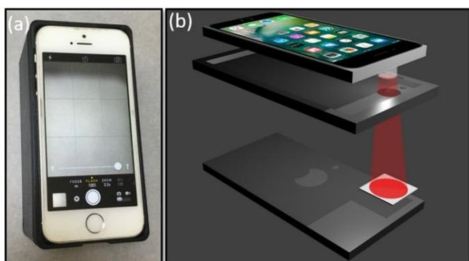
Figure 1 Smartphone biosensing system. (a) Photograph showing smartphone situated in 3D printed box. (b) Schematic illustration in a cut-away view showing, from top to bottom, the smartphone with red bandpass filter inserted in front of the smartphone LED flash, the top of the 3D printed box, the PSiM positioned below the smartphone camera, and the bottom of the 3D printed box.
