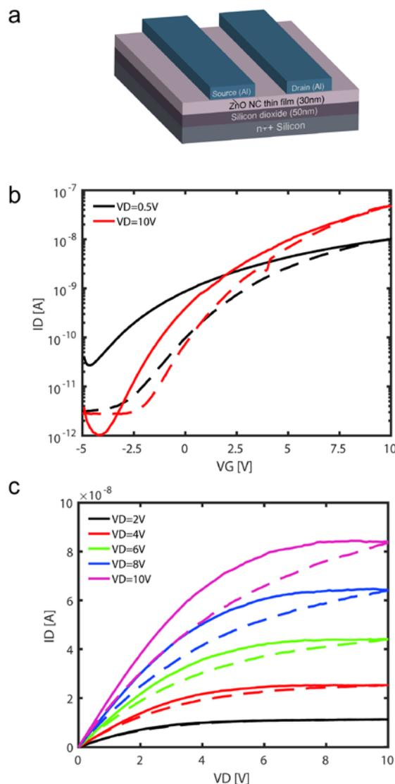
**Fig.8** (a) Structure of the back-gate, top-contact ZnO nanocrystal TFT. (b) Transfer characteristics and (c) output characteristics of a TFT utilizing the ZnO nanocrystals as the channel layer, after a  $300^\circ\text{C}$  annealing.
