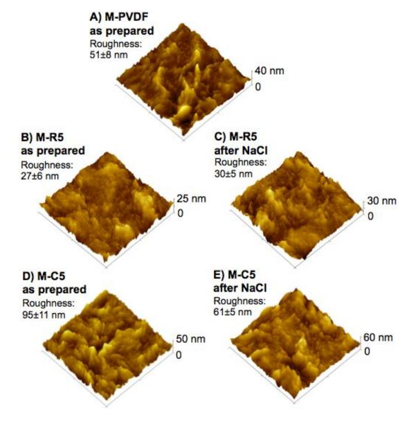
**Fig. 8** AFM images from 10 x 10  $\mu$ m<sup>2</sup> surface sections and measured surface roughness values of (A) M-PVDF as prepared, (B) M-R5 as prepared, (C) M-R5 after immersion in 0.1 M NaCl, (D) M-C5 as prepared, and (E) M-C5 after immersion into 0.1 M NaCl.
