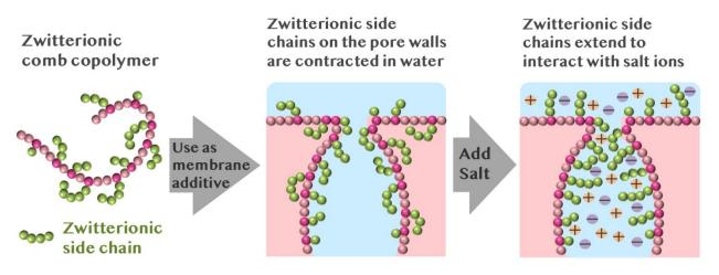
Scheme 1 Schematic showing zwitterionic comb copolymer assembly on the membrane pore walls, and the conformational rearrangement of zwitterionic side chains in response to addition of salt ions.
