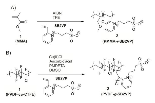
**Fig. 1** Synthesis scheme for (A) free radical polymerization (FRP) of random copolymer PMMA-*r*-SB2VP, and (B) activators regenerated by electron transfer atom transfer radical polymerization (ARGET-ATRP) of comb copolymer PVDF-*g*-SB2VP
