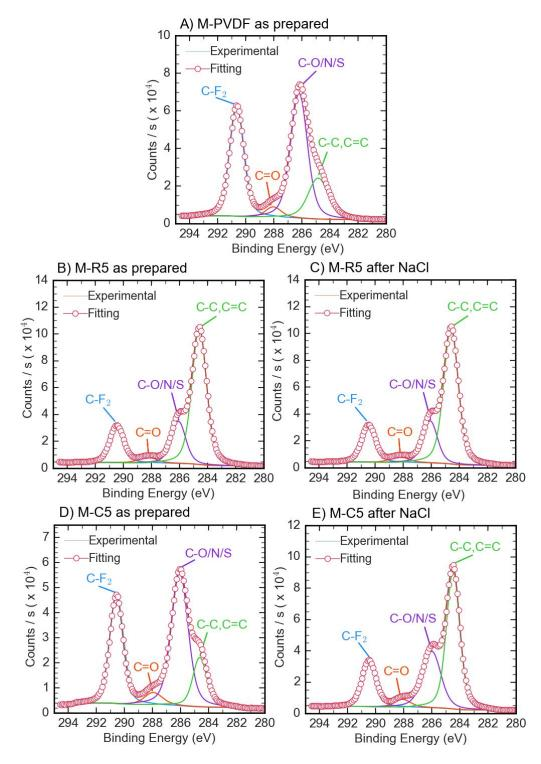
**Fig. 7** Irreversible changes on the selective layer surface chemistry of membranes due to exposure to saline solutions, characterized by XPS high resolution C 1s spectra of (A) M-PVDF as prepared, (B) M-R5 as prepared, (C) M-R5 after immersion in 0.1 M NaCl, (D) M-C5 as prepared, and (E) M-C5 after immersion into 0.1 M NaCl.
