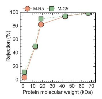
Fig. 5 Protein rejection of M-R5 and M-C5 membranes
