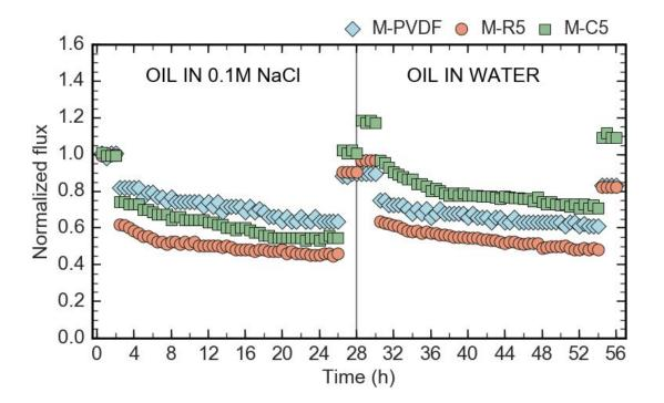
**Fig. 9** Long-term oil fouling resistance by filtration of M-PVDF (10 psi), M-R5 (5 psi), and M-C5 (10 psi) membranes. The fluxes are plotted after normalizing by the average initial flux of each membrane; 19 L/m<sup>2</sup>.h for M-PVDF, 38 L/m<sup>2</sup>.h for M-R5, and 37 L/m<sup>2</sup>.h for M-C5.
