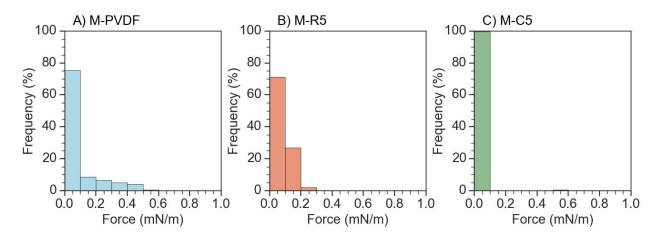
**Fig. 10** Distributions of normalized jump-to-force measurements between the AFM particle (foulant) probe and membranes (A) M-PVDF, (B) M-R5, and (C) M-C5.
