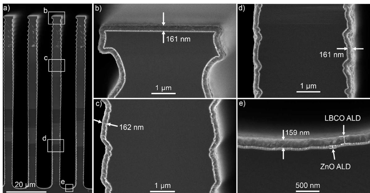
**Fig. 2** SEM images of etched Si trenches with ALD ZnO (to reduce charging and increase contrast) and LBCO showing conformality. Full trench shown in a) with locations along height of trench highlighted and shown in b-e with measured thicknesses.
