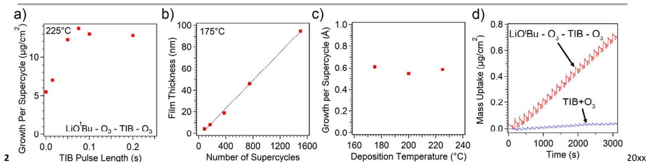
**Fig. 1** Characterization of ALD film growth with in situ QCM (a,c) and spectroscopic ellipsometry (b,d) showing a) saturation of growth rate with increasing TIB pulse time, b) linearly increasing film thickness with number of supercycles, c) dramatically enhanced growth of the LBCO ALD process compared to the binary boron oxide process, and d) consistent growth rate across a range of deposition temperatures.
