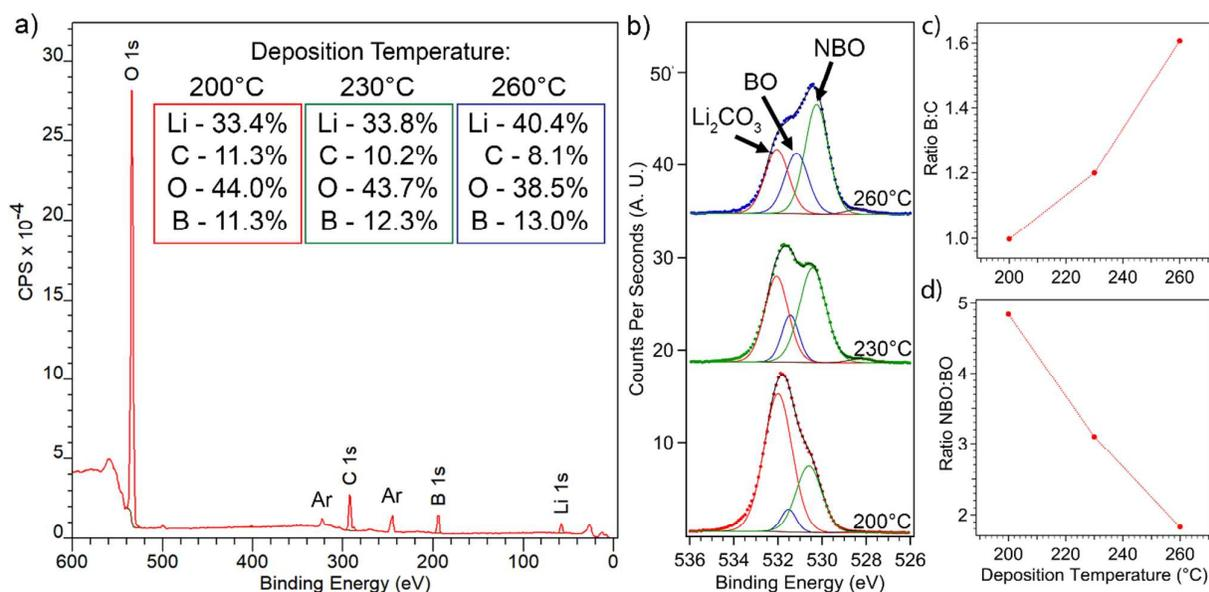
Fig. 3 a) XPS survey scan for 200°C deposition temperature with insets showing calculated compositions for each as-deposited film at the three deposition temperatures. b) XPS O 1s core scan showing changes in oxygen bonding environment with deposition temperature. c) plot of the ratio of boron to carbon and d) the ratio of non-bridging oxygen to bridging oxygen with deposition temperature. All data shown are after 15 minutes of sputtering with Ar ions to remove surface layers.
