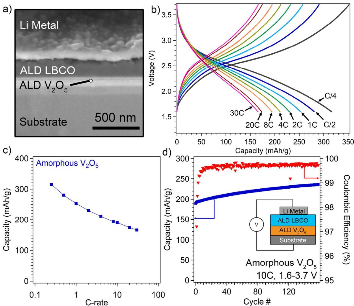
**Fig. 9** a) SEM image of FIB cross-section of full cell stack used in electrochemical measurements. b) charge and discharge curves at different rates for full cells, with schematic inset of cell architecture. c) discharge capacity at varying rates corresponding for crystalline and amorphous ALD  $\text{V}_2\text{O}_5$  cathode films d) plot of discharge capacity and coulombic efficiency for cell cycled at 10C.
