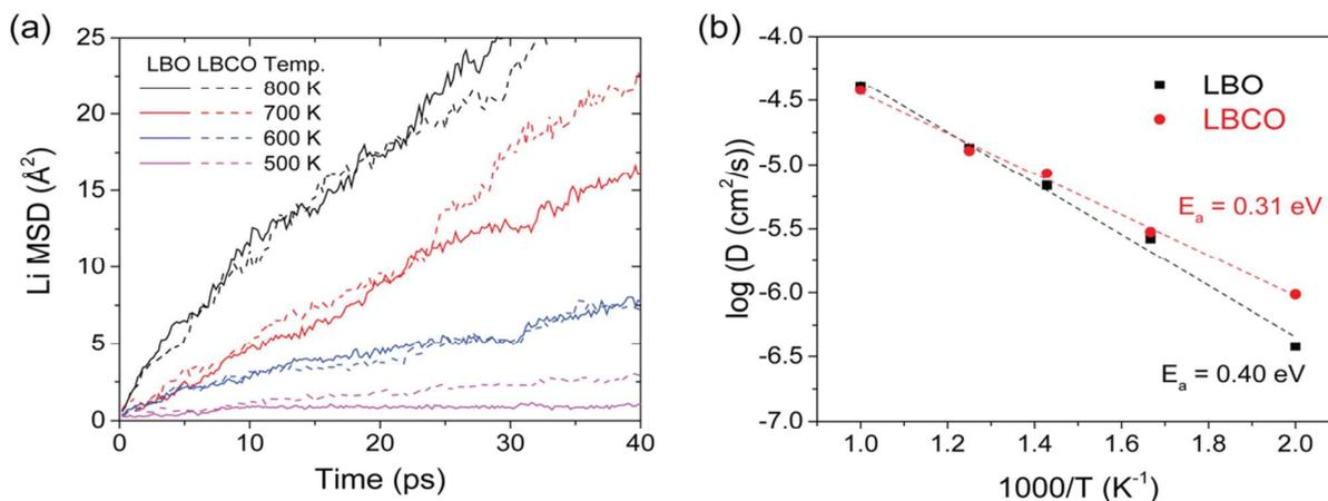
Fig. 6 Calculation of Li diffusivity in glassy LBO and LBCO: (a) Li ion MSD for  $T = 500 - 800$  K, and (b) Arrhenius plots for Li diffusivity over the temperature range  $500 - 1000$  K.
