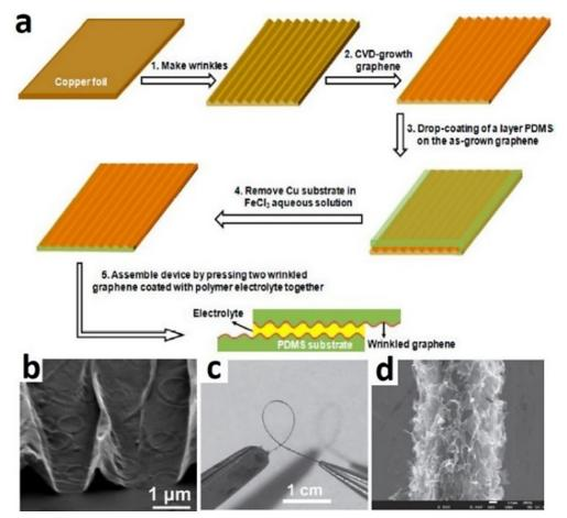
**Figure 2**. (a) Schematic illustration to fabrication procedures for transparent wrinkled graphene sheets and stretchable supercapacitors. Reproduced with permission.<sup>32</sup> Copyright 2013, American Chemical Society. (b) SEM image of buckled graphene film on PDMS substrate. Reproduced with permission.<sup>33</sup> Copyright 2014, American Chemical Society. (c) A photograph of GF@3D-G. (d) SEM image of GF@3D-G. Reproduced with permission.<sup>34</sup> Copyright 2013, Wiley-VCH.
