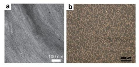
**Figure 3**. (a) TEM images of monolayer superlattice nanomembrane of ultrathin gold nanowires. Reproduced with permission.<sup>36</sup> Copyright 2012, Wiley-VCH. (b) Optical microscopy image of the gold nanowire mesh film. Reproduced with permission.<sup>35</sup> Copyright 2016, Wiley-VCH.
