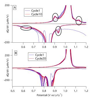
Fig. 5 Differential capacity plots of: (A) a crystalline-Sb@Cu anode and (B) a crystalline-Sb@Ni@Cu anode.
