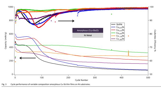
reversible capacity and cycling stability of these films. Deposition of these films onto Ni foil substrates ensures that the Sb:Cu ratio of the films stays constant during cycling, unlike Sb@Cu anodes where Cu from the substrate can diffuse into the film during cycling. Figure 3 shows the cycle lifetimes of the Cu<sub>x</sub>Sb@Ni anodes as measured by the specific delithiation capacity for each cycle.
