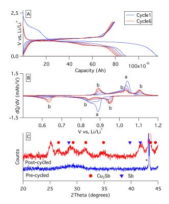
Fig. 2 Characterization of Sb@Cu anode cycled in a Li-ion battery: (A) chargedischarge curves for 6 cycles between 0.05-2 V vs. Li/Li<sup>+</sup>, (B) the corresponding differential capacity plots, (C) and ex-situ XRD before and after cycling. The Cu substrate is marked by \*.
