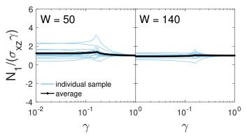
FIG. 8. Off-lattice networks show signatures of anisotropy in  $N_1$  at the critical strain, but these deviations appear to average out in the limit of large system sizes or when averaged over many samples. For 2D packing-derived networks with z=3.3 and  $\tilde{\kappa}=10^{-6}$ , we observe a decrease in the magnitude of the deviations of  $N_1$  from the Lodge-Meissner relation with increasing system size.
