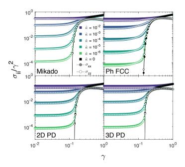
FIG. 5. Normal stress components  $\sigma_{xx}$  (closed symbols) and  $\sigma_{zz}$  (open symbols) normalized by  $\gamma^2$  for (top left) Mikado networks with z=3.3, (top right) phantom FCC networks with z=3.4, (bottom left) 2D packing-derived networks with z=3.3, and (bottom right) 3D packing-derived networks with z=4.8, all with varying  $\tilde{\kappa}$ .
