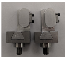
Fig. 4 Clamps developed to hold the spun UHMWPE fibers during post drawing.
