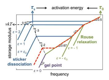
Figure 11: Stress relaxation originated from Rouse motion (green lines) and sticker dissociation (blue lines) for unentangled associative polymers, where the  $\tau_0$  corresponds to  $G' \sim v_{\text{Kuhn}}kT$  of the Rouse region, and  $\tau_s$  corresponds to the relaxation time at the full gelation point ( $\varepsilon = 1$ ) where plateau modulus  $G' \sim vkT$ . (logarithmic scales)
