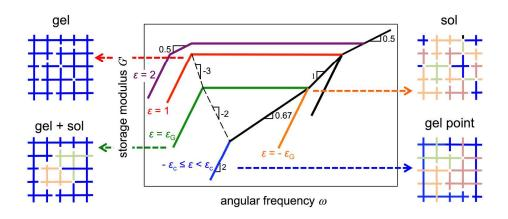
Figure 6: Schematic predicted evolution of storage modulus G' against frequency  $\omega$  along with a sol-gel transition predicted by the reversible gelation model for unentangled associative polymers.<sup>15</sup> (logarithmic scales) The unconnected chains are represented in different colors.
