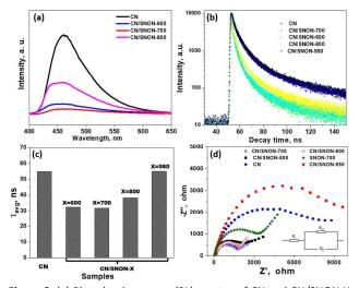
**Figure 8:** (a) Photoluminescence (PL) spectra of CN and CN/SNON-X at an excitation wavelength of 336 nm; (b) Time-resolved fluorescence emission decay curves for g-C<sub>3</sub>N<sub>4</sub> and CN/SNON-X. The emission wavelength was set at 460 nm, with the excitation wavelength at 336 nm; (c) Weighted average lifetimes ( $\tau_{avg}$ ) for g-C<sub>3</sub>N<sub>4</sub> and heterojunctions CN/SNON-X; (d) Electrochemical impedance spectra (EIS) of photocatalysts studied.
