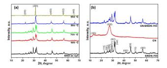
**Figure 1**: (a) PXRD patterns of SNO and different SNON-X. (b) The PXRD pattern of  $C_3N_4$  and heterojunctions based on  $C_3N_4$  and SNON-700 (\* represents the peaks due to oxynitride phase which appears as low as 800 °C).
