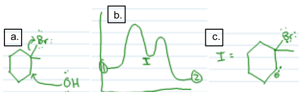
Fig. 10 Anton's (a) proposed mechanism for Reaction 2; (b) re-drawn RCD IB showing that Reaction 2 proceeds through an intermediate (label “I” under the valley); (c) proposed intermediate structure.
