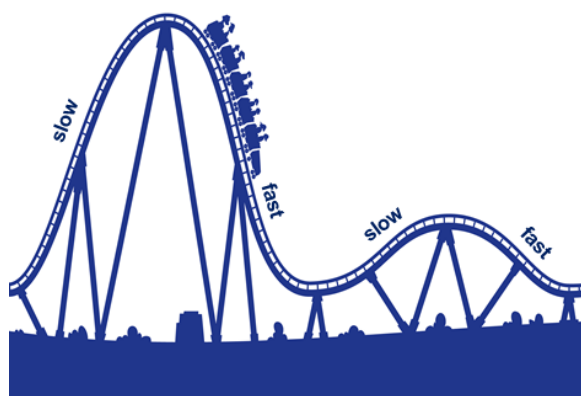
Fig. 6 Changes in the speed of a roller coaster. (Adapted from Clipartix.com, n.d.)
