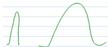
Fig. 7 Arina’s drawing to explain that more narrow peaks indicate faster reactions (left) while wider peaks indicate slower reactions (right).
