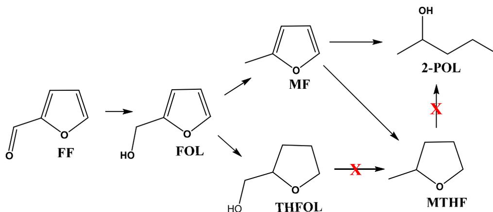
**Scheme 1.** Single-step catalytic conversion of FF to 2-POL.
