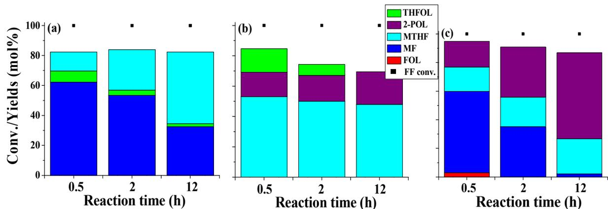
**Figure 3.** FF conversion and product yields on Al<sub>2</sub>O<sub>3</sub> supported bimetallic (a) Cu-Ni, (b) Co-Ni, (c) and Cu-Co catalysts. All reactions were run with an FF loading of 1 g, a catalyst loading of 0.3 g, 25 mL of 1,4-dioxane as a solvent, a temperature of 240 °C, and an H<sub>2</sub> pressure of 35 bar.
