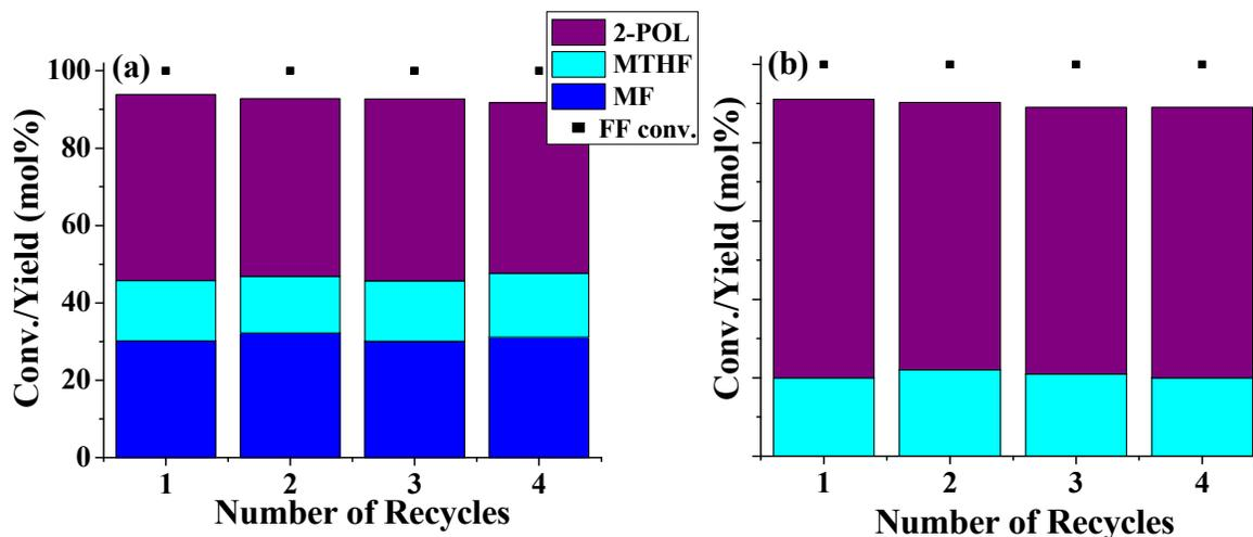
**Figure 4.** FF conversion and product yields as a function of number of catalyst recycles for Cu-Co/Al<sub>2</sub>O<sub>3</sub> catalysts recycled after (a) 2 h and (b) 12 h reaction time. Reaction conditions were a FF loading of 1 g, catalyst loading of 0.3 g, 25 mL of 1,4-dioxane as a solvent, a temperature of 240 °C, H<sub>2</sub> pressure of 45 bar.
