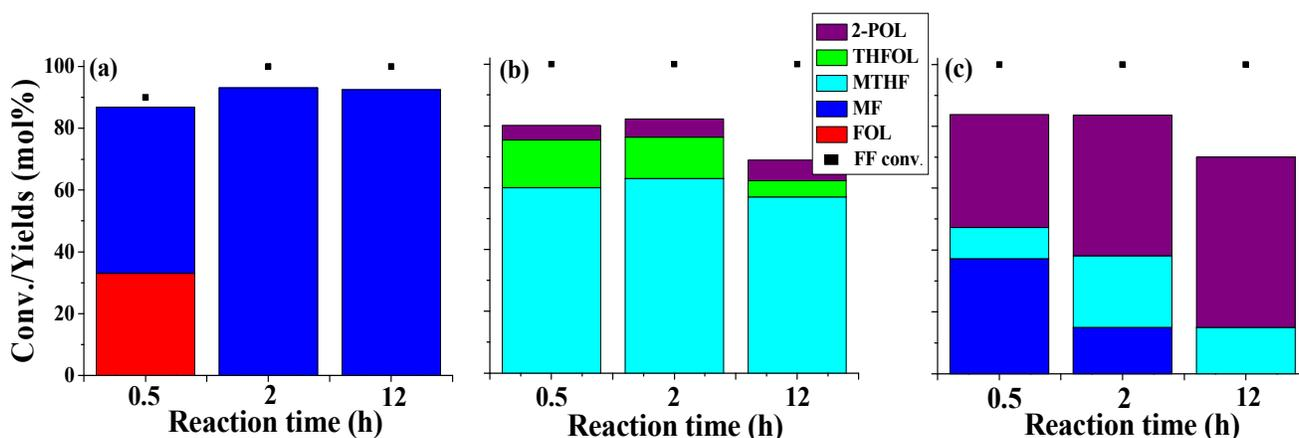
**Figure 2.** FF conversion and product yields on monometallic (a) Cu, (b) Ni, and (c) Co on Al<sub>2</sub>O<sub>3</sub> catalysts. All reactions were run with a FF loading of 1 g and catalyst loading of 0.3 g in 25 mL of 1,4-dioxane as a solvent at temperature of 240 °C for 0.5-12 hours and an H<sub>2</sub> pressure of 35 bar.
