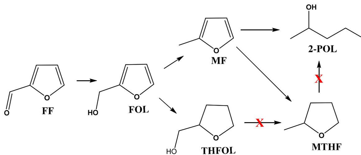
**Graphical Abstract:** Catalytic conversion of furfural to 2-pentanol over Co-Cu/Al<sub>2</sub>O<sub>3</sub> catalysts
