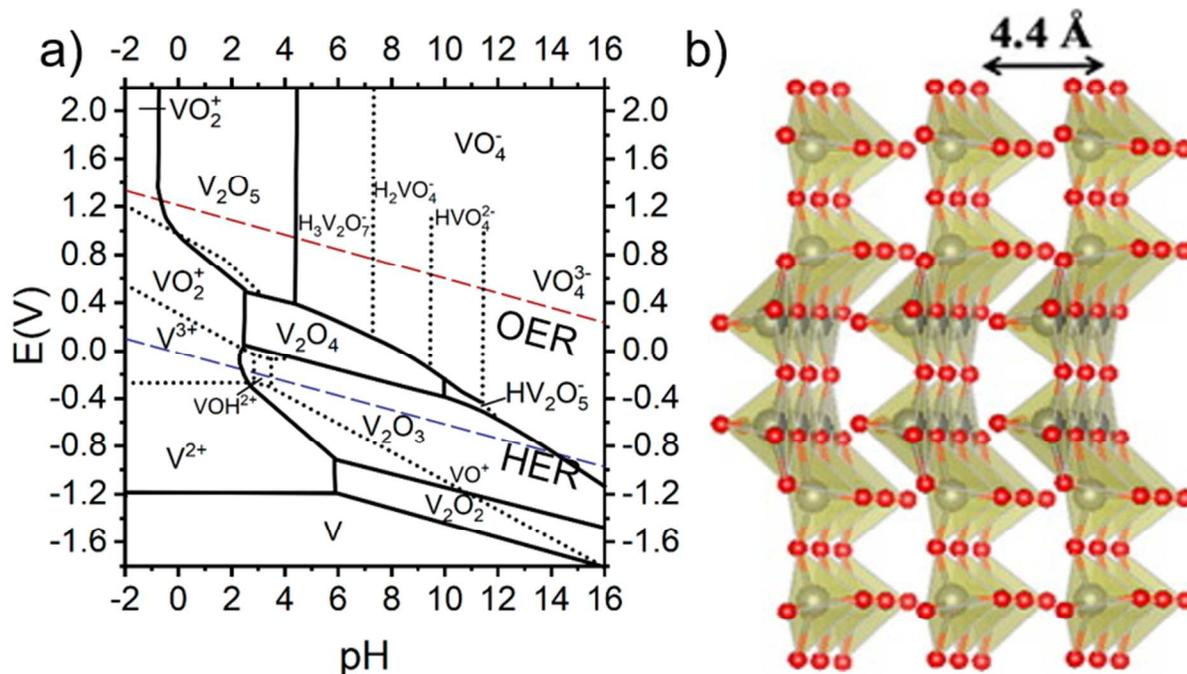
**Figure 9.** a) Pourbaix diagram of V<sub>2</sub>O<sub>5</sub> in water (adapted from Ref. 25), b) Crystal structure of α-V<sub>2</sub>O<sub>5</sub>. Adapted with permission from Ref. 101. Copyright 2016 American Chemical Society.
