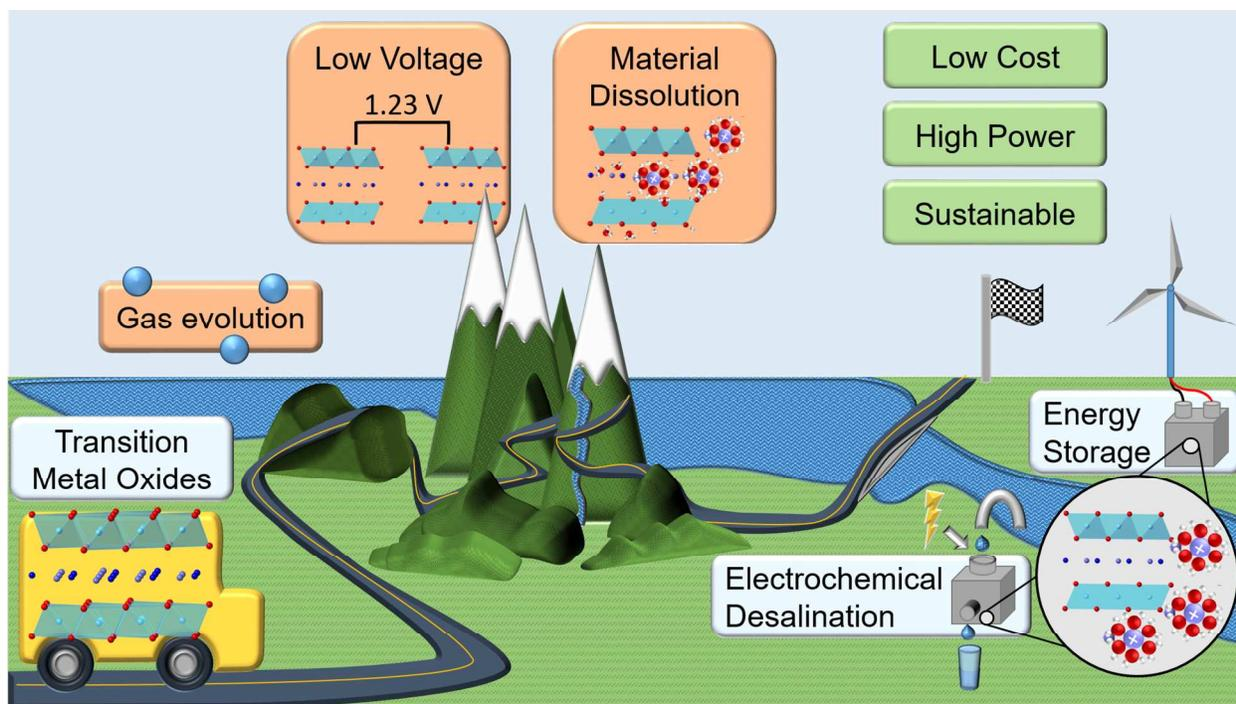
**Figure 1.** Overview of the challenges and benefits of transition metal oxides for aqueous  $\text{Na}^+$  electrochemical energy storage.
