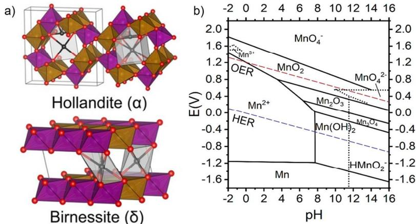
**Figure 6.** a) The crystal structures of  $\alpha$ -MnO<sub>2</sub> and  $\delta$ -MnO<sub>2</sub>, two polymorphs of MnO<sub>2</sub> that are capable of bulk intercalation of Na<sup>+</sup>; the Na<sup>+</sup> intercalation sites are indicated by the gray polyhedra. Adapted with permission from Ref. 46. Copyright 2017 American Chemical Society. b) The Pourbaix diagram of MnO<sub>2</sub> in water (adapted from Ref. 25).
