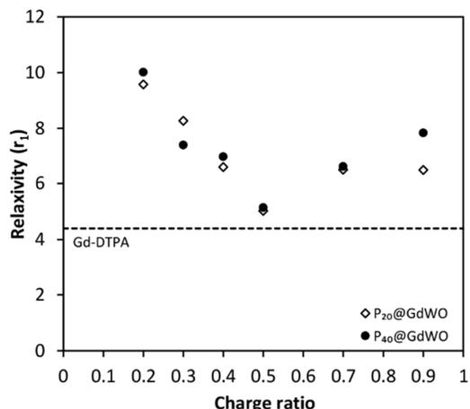
Figure 4 Relaxivity measurements of the  $P_{20}@GdWO$  and  $P_{40}@GdWO$  nano-assemblies at different charge ratios. The dotted line represents the  $r_1$  of Gd-DTPA.
