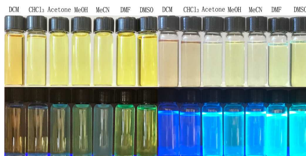
Fig 2. Solvatochromism of 1mM 1a (top left: under sunlight; bottom left: under 365nm UV light) and 1b (top right: under sunlight; bottom right: under 365nm UV light) in a set of solvents.
