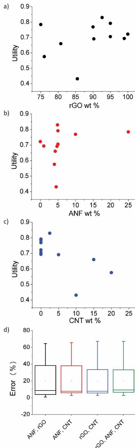
Figure 3. Values of utility for the features (a) GO wt %, (b) ANF wt %, and (c) CNT wt % for each experimental data point. (d) Leave-one-out cross validation error of four different feature sets. Boxes ; are a statistical representation of the distribution of errors for each feature set. The top and bottom line are the maximum and minimum data points, the top and bottom of the box are the 75th and 25th percentile markers, the middle line is the median, and the point within the box is the mean.
