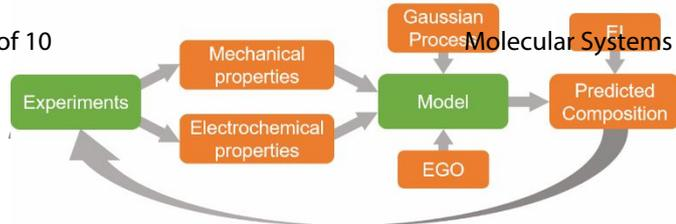
Figure 3. Schematic showing feedback between experimental data and the computational model. EI is expected improvement and EGO is efficient global optimization.
