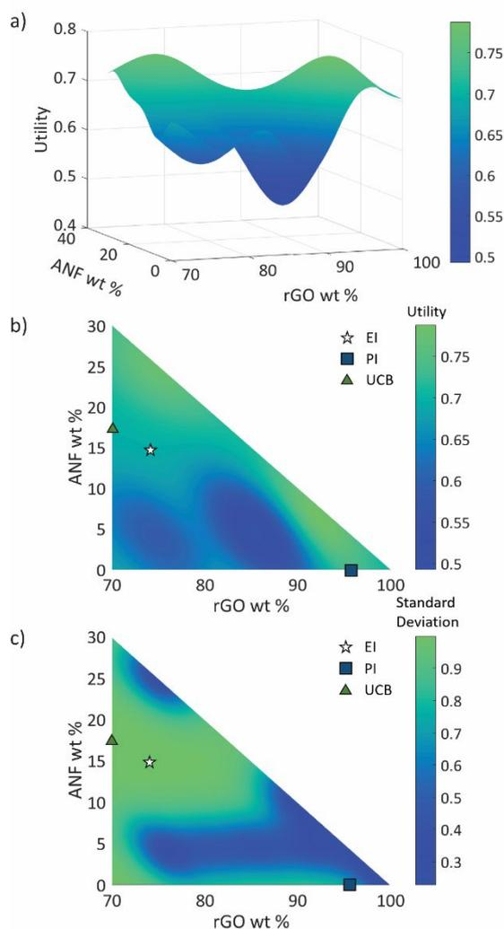
Figure 4. Three-dimensional plot of (a) utility, and (b) contour plots of utility and (c) standard deviation vs. composition. Circular points represent initial experimental data while the star, square, and triangle represent recommendations from the model based on either expected improvement (EI), probability of improvement (PI), or upper confidence bound (UCB), respectively.
