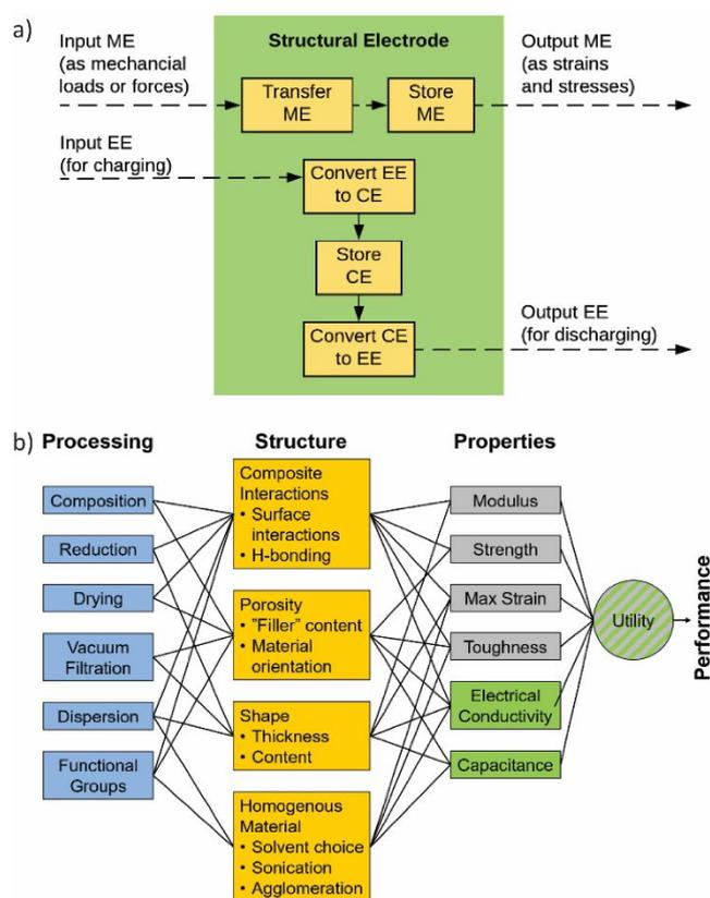
Figure 1. (a) Component level functional diagram of a typical structural electrode where ME is mechanical energy, EE is electrical energy, and CE is chemical energy. In this diagram, the structural electrode can discharge electrical energy while also safely handling mechanical loads. (b) Material level system chart of the interactions between process, structure, and properties within a composite electrode consisting of ANFs, graphene, and CNTs.
