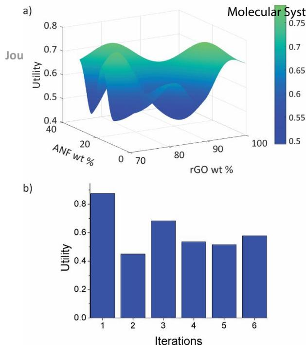
Figure 5. (a) Predicted utility function after 6 iterations and (b) utility of samples with composition predicted by EI at each iteration.
