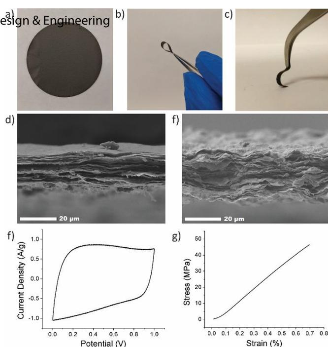
Figure 4. Digital images of (a) an rGO electrode and (b-c) an rGO/ANF composite electrode (no CNTs). Cross-sectional SEM images of (d) an rGO/ANF electrode without CNTs (95/5 wt % rGO/ANF) and (e) with 20 wt % CNTs (76/4/20 wt % rGO/ANF/CNTs). (f) A representative cyclic voltammogram and (g) a typical stress-strain curve for an rGO/ANF/CNT composite electrode (90.25 rGO wt %, 4.75 ANF wt %, 5 CNT wt %).
