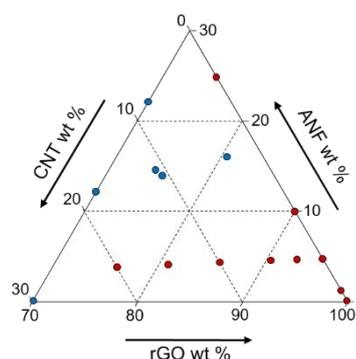
Figure 2 Ternary diagram describing the design space for rGO/ANF/CNT supercapacitor electrodes. Original experimental data are plotted with red circles while predicted compositions which were then validated experimentally are plotted with blue circles.
