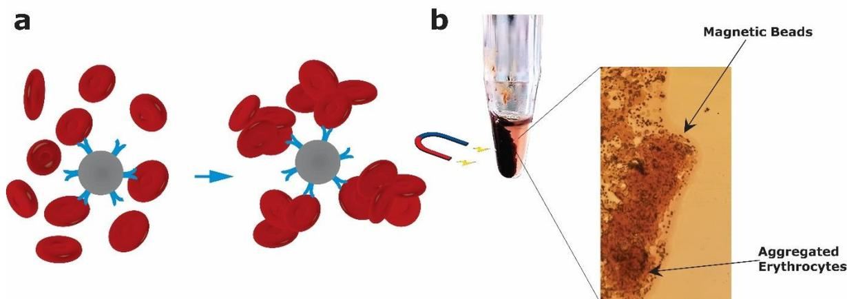
**Figure 2:** a) Effect of aggregation of blood cells prior to capture and b) Separation of plasma from captured red blood cells with application of a magnetic field as seen under a microscope
