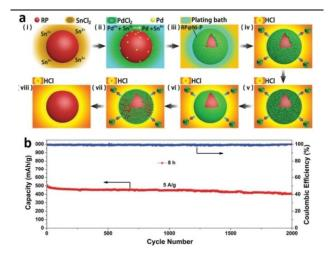
**Fig. 7** Schematic illustration of electroless deposition of Ni on an RP nanoparticle (a(i–iii)) and the evolution of the RP@Ni–P core@shell nanostructure through chemical dealloying (a(iv–viii)); (b) Long-term cycling performance of the 8 h RP@Ni–P electrodes at 5 A/gcomposite between 0.05 and 2.0 V. Reproduced with permission. Reprinted from ref 111 with permission from the Royal Society of Chemistry.
