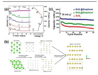
Fig. 16 (a) Ex-situ XRD patterns of the SnS@graphene electrode collected at various points as indicated in the corresponding voltage profile; (b) Schematic illustration of the structural evolution of orthorhombic-SnS and hexagonal-SnS<sub>2</sub> during the sodiation; (c) Cycling performances of SnS@graphene, SnS<sub>2</sub>@graphene, and SnS<sub>2</sub> electrodes. Reprinted from ref 43 with permission from American Chemical Society.
