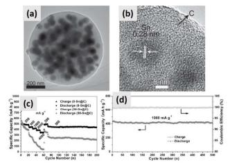
**Fig. 4** (a) Transmission electron microscope (TEM) image and (b) high resolution TEM (HRTEM) image of 8-Sn@C; (c) Rate capability of the 8-Sn@C and 50-Sn@C electrodes in the voltage range of 0.01 to 2.0 V, and (d) long-term cycling stability of the 8-Sn@C electrode in the same voltage range at a current density of 1 A/g. Reprinted from ref 17 with permission from John Wiley and Sons.
