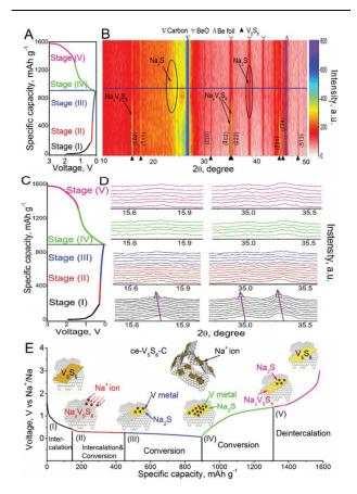
**Fig. 15** Charge–discharge profiles (A and C), the corresponding contour plots (B), and selected  $2\theta$  region plot (D) from the in situ XRD results at different discharge/charge states of the ce-V<sub>5</sub>S<sub>8</sub>–C hybrid anodes, and a schematic illustration of the energy storage mechanism of the ce-V<sub>5</sub>S<sub>8</sub>–C hybrid anode at different stages (E). Reproduced with permission. Reprinted from ref 215 with permission from The Royal Society of Chemistry.
