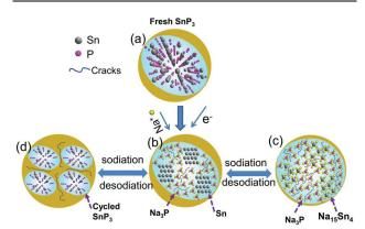
Fig. 9 Schematic illustration of the sodiation and desodiation of  $SnP_3/C$  composite. The yellow outer layer denotes carbon. Reproduced with permission. Reprinted from ref 125 with permission from John Wiley and Sons.
