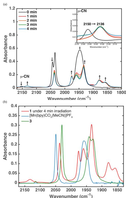
**Fig. 8** IR spectral changes upon photolysis of 20 mM **1** (a) in MeCN with 365 nm LED light (see experimental section for details). Changes of cyanide (inset) and carbonyl stretching bands are indicated with arrows. (b) The IR spectrum upon 4 min irradiation of **1** (blue trace in Fig. 8a) is compared with that of **3** and  $[\text{Mn}(\text{bpy})\text{CO}_3(\text{MeCN})]\text{PF}_6$  (keeping all the other conditions fixed).
