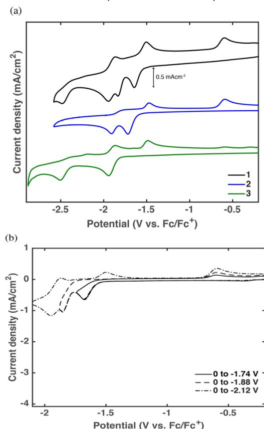
**Fig. 3** (a) CV data of complex 1-3 (1mM) using 0.1 M TBAP in MeCN under Ar-atmosphere at 250 mV/s using a 3 mm glassy carbon working electrode, a platinum foil counter electrode and a  $\text{Ag}/\text{Ag}^+$  non-aqueous reference electrode. All potentials are referenced to  $\text{Fc}/\text{Fc}^+$ . (b) CV data of complex 1 at various switching potentials using a scan rate of 250 mV/s. Other conditions are the same as Fig. 3a.
