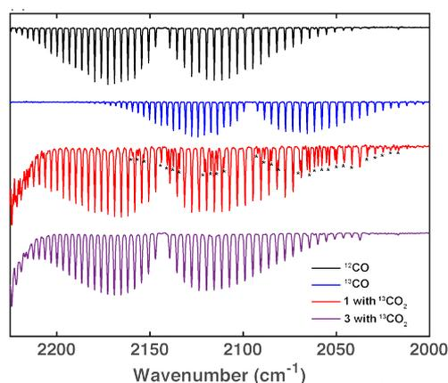
Fig. 9. FT-IR spectra of standard samples of <sup>12</sup>CO (black trace) and <sup>13</sup>CO (blue trace) to our headspace samples (red and purple traces for **1** and **3**, respectively); see experimental section for details. In case of **1**, the headspace sample yields a mixture of <sup>12</sup>CO and <sup>13</sup>CO (black stars), while the sample from **3** contains only <sup>12</sup>CO.
