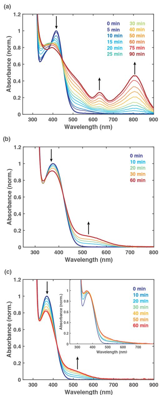
**Fig. 7** Evolution of UV-Vis absorption spectra of (a) **2** and (b) **3** in stirred MeCN at 298 K upon irradiation with a 365 nm pulsed laser. (c) Photoresponse of **1** in MeCN and 2-MeTHF (inset), respectively, and all the other experimental conditions are kept fixed.
