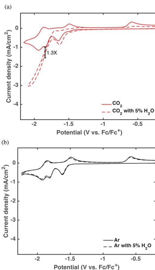
**Fig. 4** CV data of complex 1 with and without 5%  $\text{H}_2\text{O}$  under  $\text{CO}_2$  atmosphere (a) and Ar atmosphere (b) at a scan rate of 250 mV/s. All other conditions are the same as given in Fig. 3.
