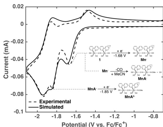
Fig. 6 Comparison of simulated and experimental CV data of complex **1** using 0.1 M TBAP in MeCN under Ar-atmosphere at a scan rate of 250 mV/s. A 3 mm glassy carbon electrode was used as a working electrode. In the simulations, we excluded any data more positive than -0.9 V vs Fc/Fc<sup>+</sup>. The reductive features are described in the text.
