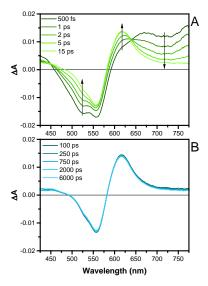
Figure 7. Excited-state absorption difference spectra of 2 in dichloromethane following 550 nm pulsed excitation (105 fs fwhm).
