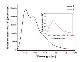
Figure 5. Photoluminescence spectra of optically matched solutions of 1 and 2 at room temperature in dichloromethane (OD = 0.1 at 500 nm). Low temperature
