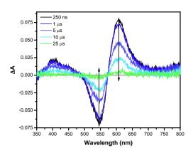
**Figure 8**. Excited-state absorption difference spectra of **2** in dichloromethane following 530 nm pulsed excitation (7 ns fwhm). The sample was deaerated using the freeze-pump-thaw method.
