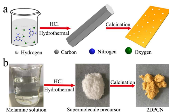
Scheme 1. (a) Preparation process of 2DPCN; (b) Photos of melamine solution, supramolecular precursor and 2DPCN.
