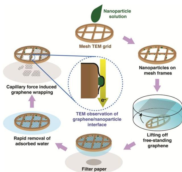
**Scheme 1** Preparation of TEM sample that expose nanocrystal/graphene interface parallel to the electron beam.
