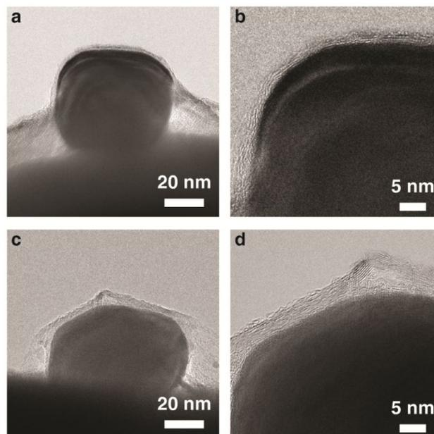
**Fig. 3** TEM images of the graphene tent which covers an Ag nanocrystal standing on the solid substrate. (a,b) TEM images of the curved conformal graphene tent with 4 to 5 layers. (c,d) TEM images of the kinked graphene tent with 18 layers. Panels (b) and (d) are magnified view of curved corner in panel (a) and kinked corner in panel (c), respectively.
