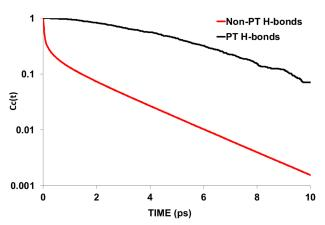
Figure 13. The continuous H-bond lifetime autocorrelation function for all protons that transferred from their original covalently bonded O1 versus all those that never transferred.
