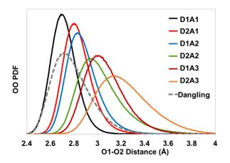
Figure 4. O1-O2 pair distribution functions showing longer distances with higher rank protons. Short distance tail on D1A1 presages more likely proton transfer for these protons.
