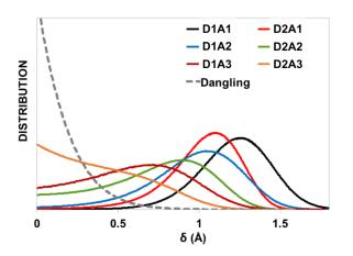
Figure 6. The  $\delta$  distributions showing the difference in r3-r2 distances and the linear (large  $\delta$  distributions) versus bifurcated bonds (low  $\delta$  distributions). ). While qualitative, one could arbitrarily separate the types of bonds using a cutoff of 0.9Å, with  $\delta$  for bifurcated bonds < 0.9Å and for linear bonds > 0.9Å.
