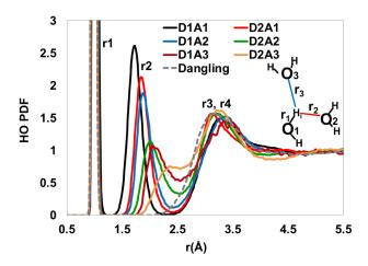
Figure 2. The HO pair distribution functions for each labeled rank in the system showing differences in the hydrogen bond distances (r2) for the ranks and similar distances for the r3 and r4 distances (distance between a proton and its  $3^{rd}$  and  $4^{th}$  O neighbors). Inset shows the H<sub>i</sub> and O labels and r1, r2, and r3 distances.
