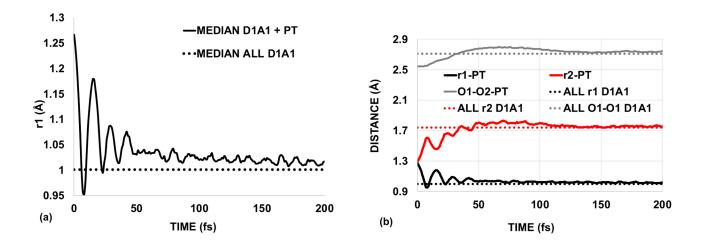
Figure 11. (a) Median r1 covalent bond length for all D1A1 (dotted line) and all D1A1 that showed auto dissociation via proton transfer, PT (the latter as a function of time prior to the PT event, which occurred at time=0). (b) Median r1, r2 (H-bond length) and O1-O2 distance for all D1A1 (dotted lines) and for all D1A1 that showed PT (the latter as a function of time prior to the PT event, which occurred at time=0).
