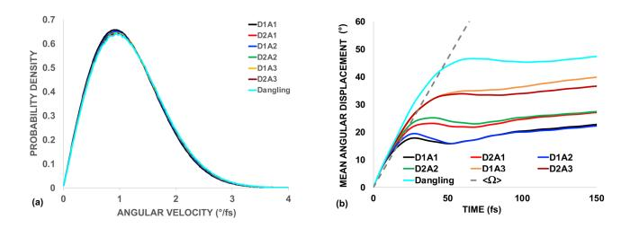
Figure 10: (a) Distributions of instantaneous angular velocities of protons about their covalent oxygens, by rank. A slight rank-dependence exists, with a difference between bonding and dangling protons, leading to the conclusion that librational rotation rates are weakly dependent of hydrogen bond strength. (b) Mean angular displacements by rank; the dashed line represents the angular displacement of a proton rotating freely at the modal angular velocity. The intersection of this line with
