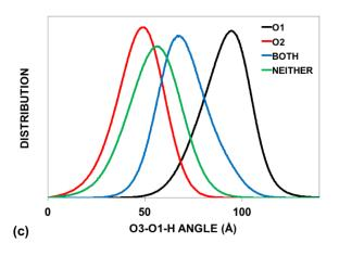
Figure 5. (a) O2-O1-H bond angles showing most protons have bond angles less than ~30°, fitting one common geometrical criterion for the hydrogen bond; (b) O3-O1-H bond angle with dual peaks determined by the relationship between O3 and O1 or O3 and O2, as shown in (c) which shows the O3-O1-H angle for O3 bonded to O1 or O2 or both or neither and a lower peak for O3 H-bonded to O2 than for O3 H-bonded to O1.
