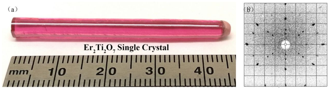
Fig. 5. (a) Image of the \text{Er}_2\text{Ti}_2\text{O}_7 crystal grown by the TSFZ technique, and (b) corresponding Laue diffraction pattern.
