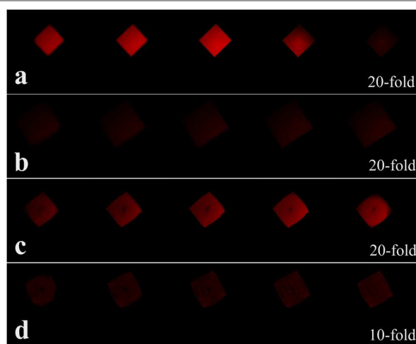
Figure 4. Laser scanning confocal microscopy (LSCM) z-stacks for (a) \text{LC}^{\text{ethanol}}@\text{CLLC} , (b) the sample in panel a after LC release, (c) \text{LC}^{\text{DMSO}\&\text{ethanol}}@\text{CLLC} , and (d) the sample in panel c after LC release. For (a), (b) and (c) the 30 \mu\text{m} z-stack was taken in the middle of the crystal at 7.5 \mu\text{m} intervals. For (d), the 56 \mu\text{m} z-stack was taken in the middle of the DMSO-expanded crystal at 14 \mu\text{m} intervals. 60 minutes in DMSO and anhydrous ethanol mixed solution ( V_{\text{DMSO}}:V_{\text{ethanol}} = 9:1 ) was used for LC release here. All samples were excited with a 405 nm diode laser.
