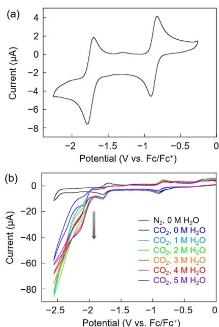
**Fig. 2** (a) CV of **Co(II)BIPC** (0.5 mM) in dry DMF with 0.1 M  $\text{TBAPF}_6$  under an  $\text{N}_2$  atmosphere. (b) CVs of **Co(II)BIPC** (0.5 mM) in dry DMF containing 0.1 M  $\text{TBAPF}_6$  under  $\text{N}_2$  (black) and  $\text{CO}_2$  with various concentrations of  $\text{H}_2\text{O}$  (from blue to purple):  $[\text{H}_2\text{O}] = 0, 1, 2, 3, 4,$  and  $5$  M. Scan rate:  $100$   $\text{mV}\cdot\text{s}^{-1}$ .
