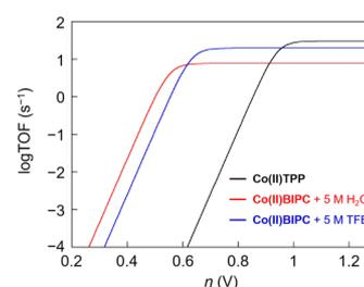
**Fig. 4** Tafel plots of **Co(II)TPP** (black), **Co(II)BIPC** with 5 M H<sub>2</sub>O (red) and **Co(II)BIPC** with 5 M TFE (blue).
