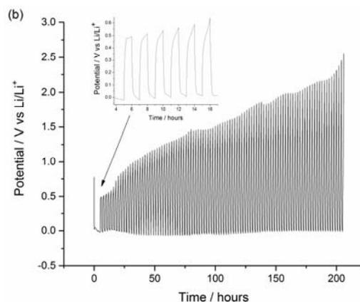
Figure 3. (a) The cyclic voltammogram of [C<sub>2</sub>epyr][Li][FSI]<sub>2</sub> at room temperature - the arrows show the direction of peak progression from the 1st to the 3rd scan, (b) cycling of the [C<sub>2</sub>epyr][Li][FSI]<sub>2</sub> over 100 cycles at a current density of 0.5 mA cm<sup>-2</sup>. With platinum working electrode (2.0 mm<sup>2</sup> surface area), a lithium strip as a quasi-reference electrode and a coiled lithium metal strip as counter electrode.
