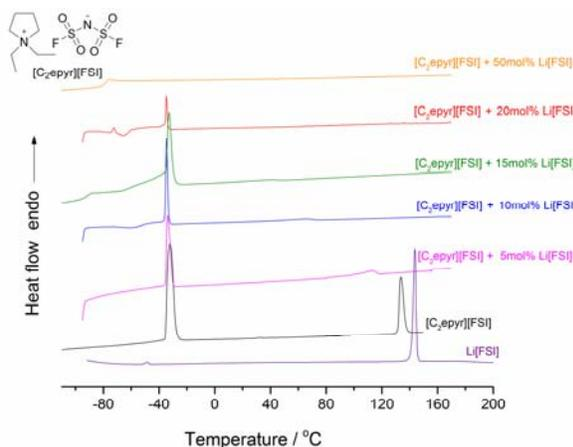
Figure 1. The DSC traces of  $[C_2\text{epyr}][\text{FSI}]$  with increasing concentration of  $\text{Li}[\text{FSI}]$ . Inset: the structure of  $[C_2\text{epyr}][\text{FSI}]$ .
